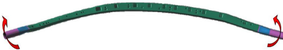
Figure 7: Spring-back approaching 10mm (0.4 in) at each end on a part 2000mm (6.5 ft) in length
