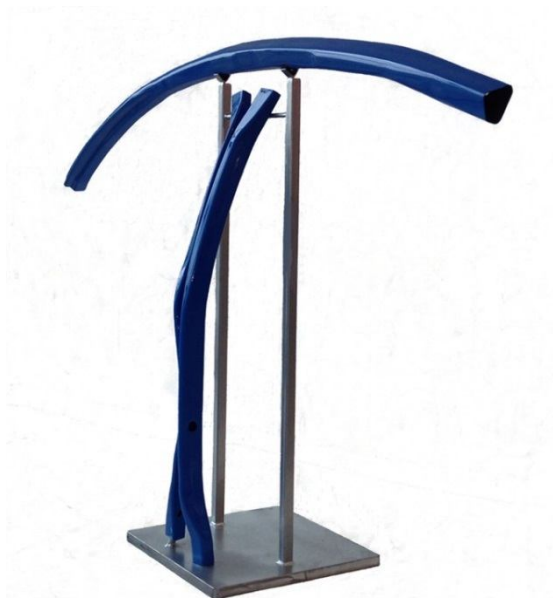
Figure 5: Hydroformed DP1000 roof rail and B-pillar for the 2013 Ford Fusion
