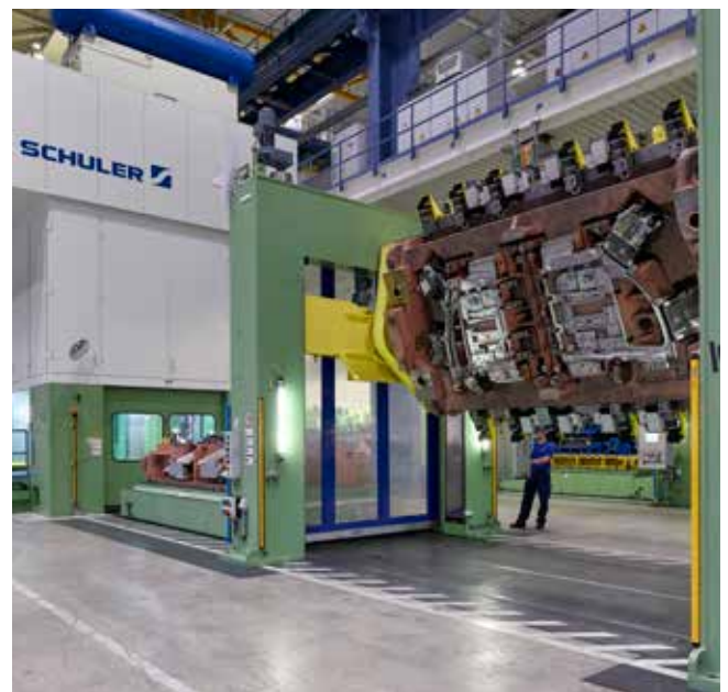
Die openers for ergonomic machining of the upper die.
