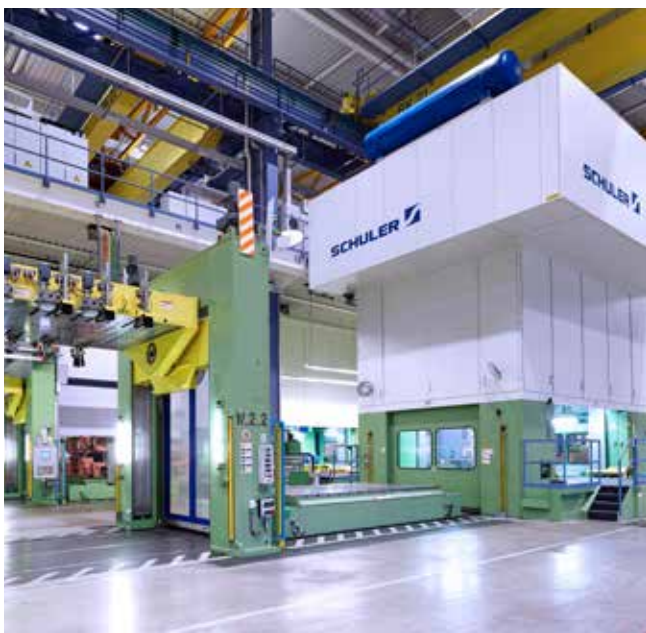
Tryout centers make the die tryout process highly efficient.
