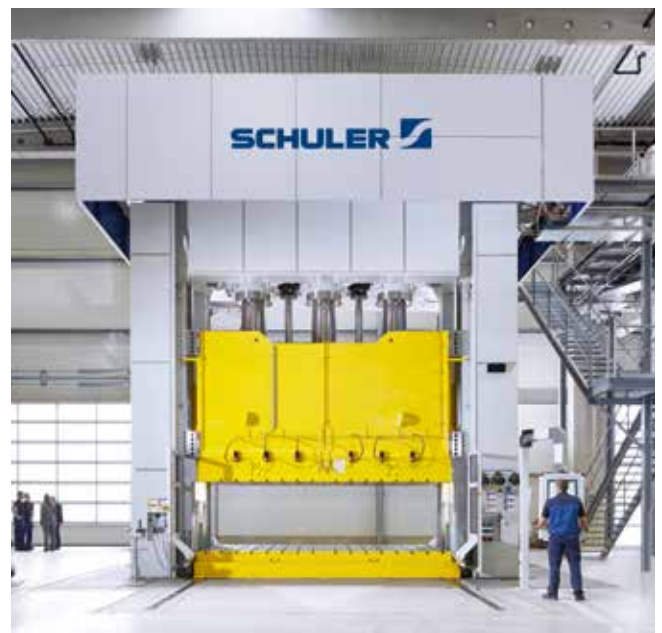
Hydraulic tryout presses enable quick tryout for draw dies.
