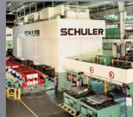
Transfer press with tri-axis transfer.
