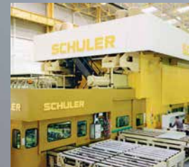
Transfer press with suction-cup tooling.
