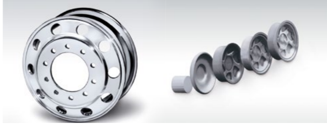
Forged truck wheel with tool sequence for aluminum wheels
