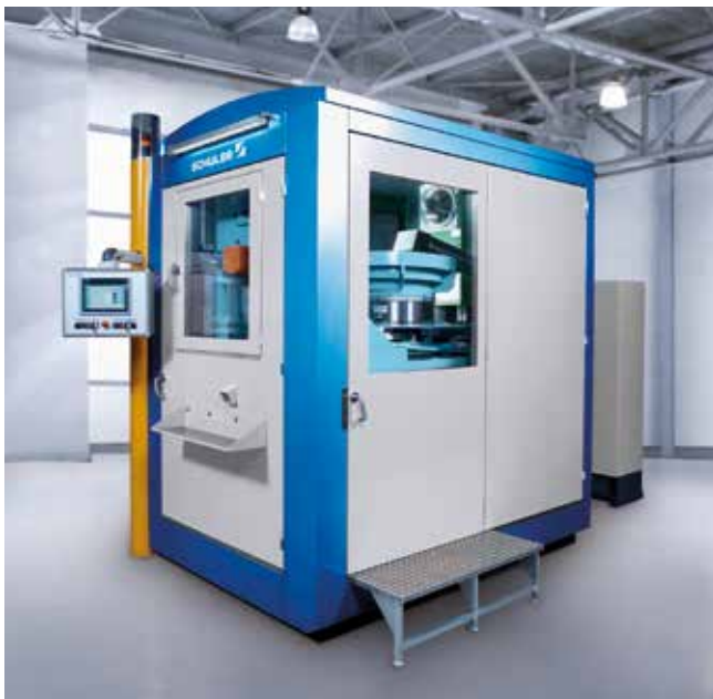
EMKH 300 with sound enclosure for further processing of the disc blanks.
