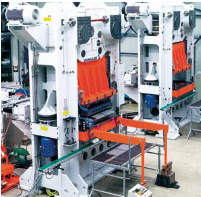
RMK 1500 radiator press with double knuckle-joint upper drive.
