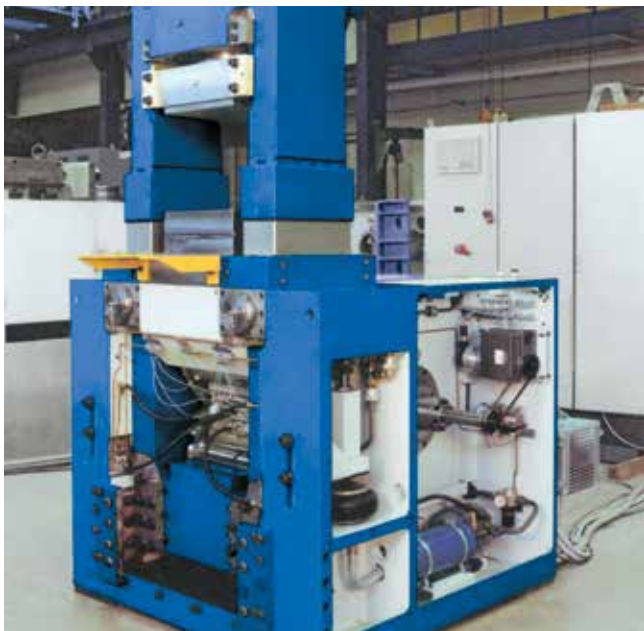
EMK 630 with knuckle-joint bottom drive.
