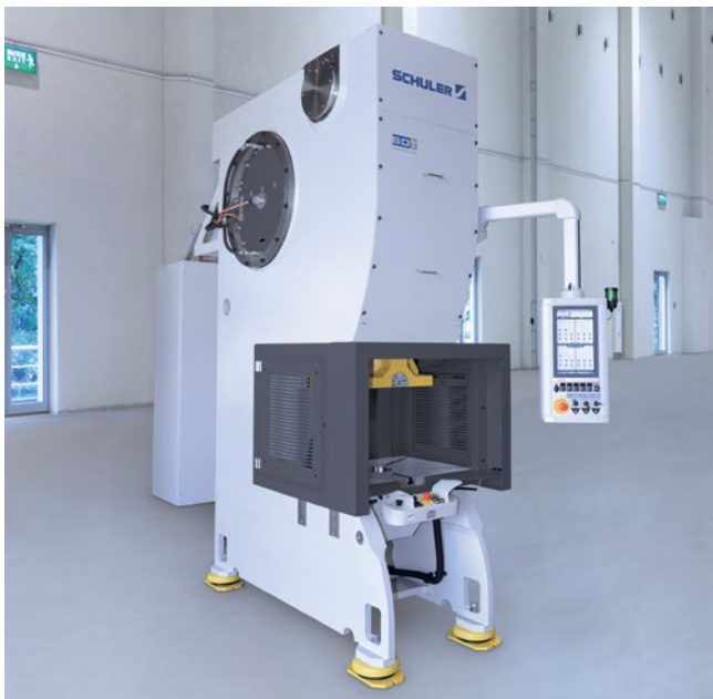
Stamping press CSC 100 with five preprogrammed slide movement curves for blanking, embossing, bending, drawing and forming.
