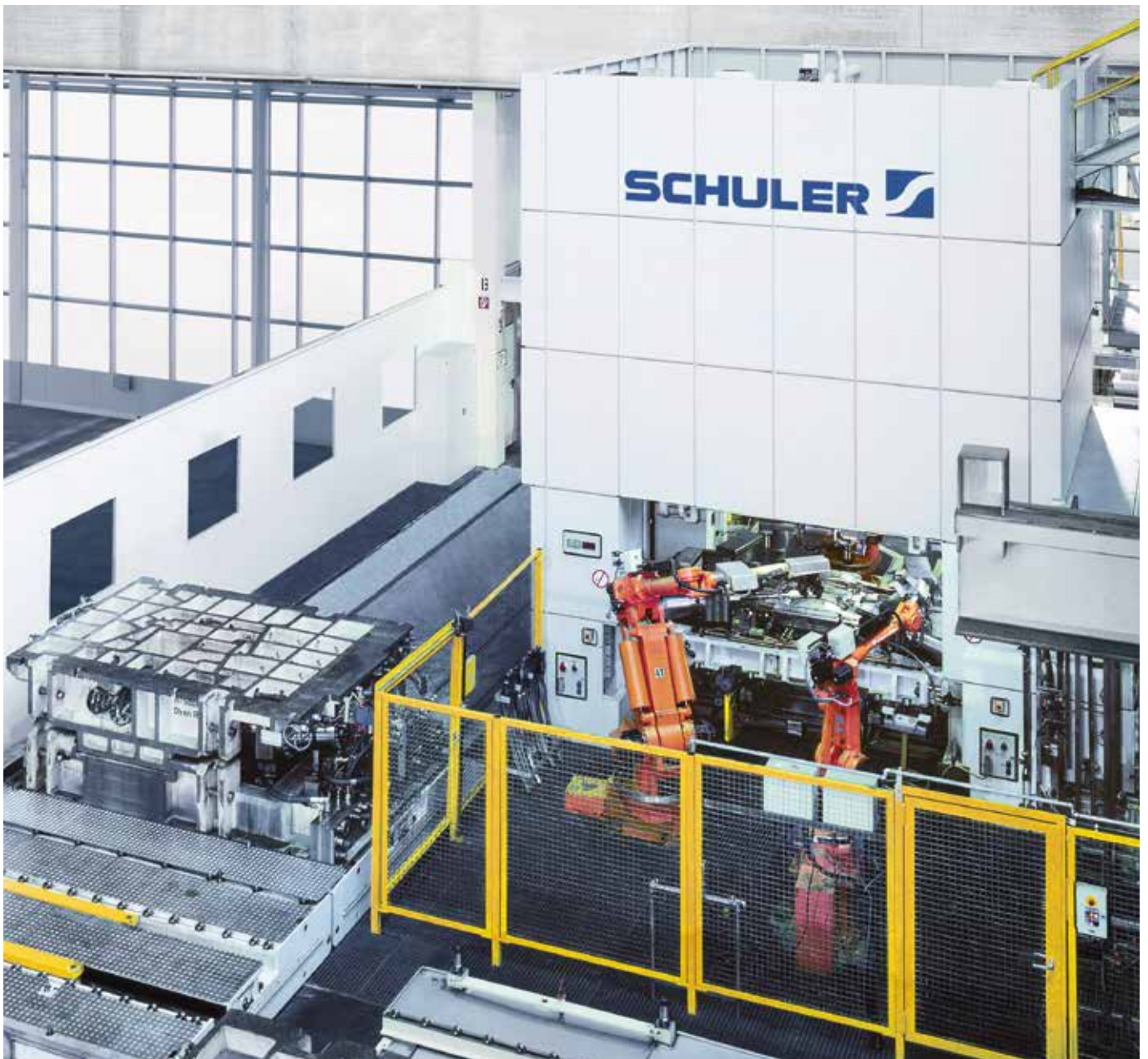
Fully automatic tubular hydroforming system at a German automobile manufacturer.
