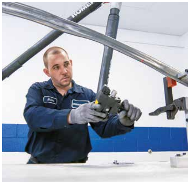
Laser scanning in part development.
