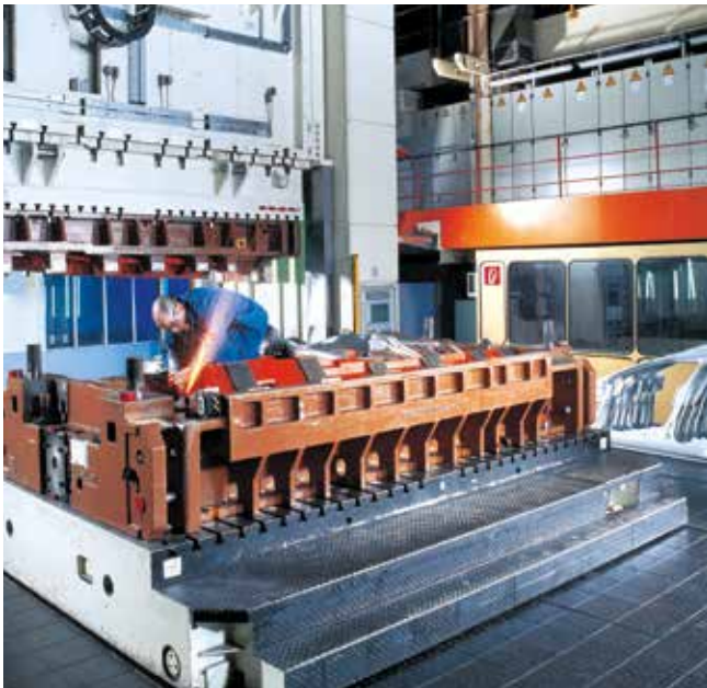
Moving bolsters for easy die change.
