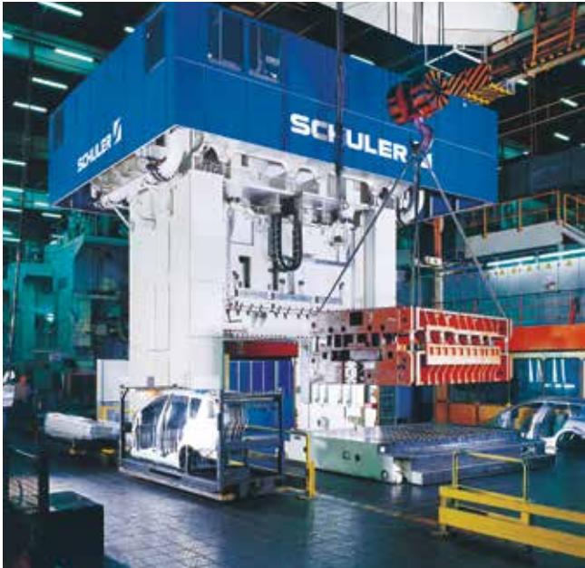
Multicurve tryout press for simulating all press types.
