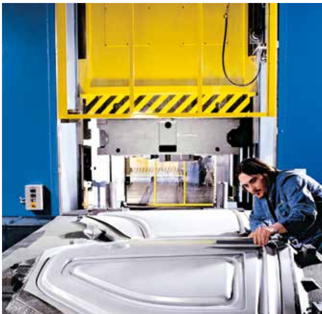
Modern tryout systems enable die start-ups in production-like conditions.
