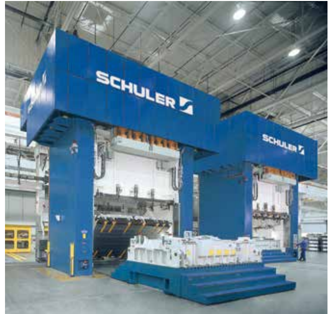
Multicurve tryout presses with rotating slide plate and moving bolster.
