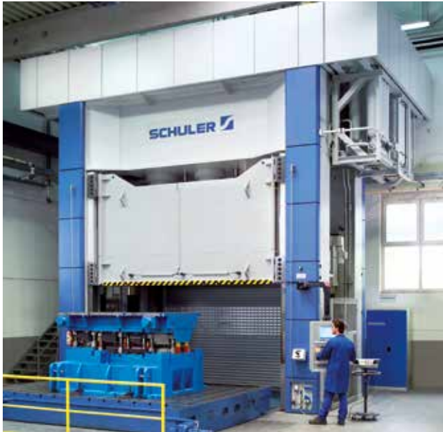
Hydraulic tryout presses in the die shop.
