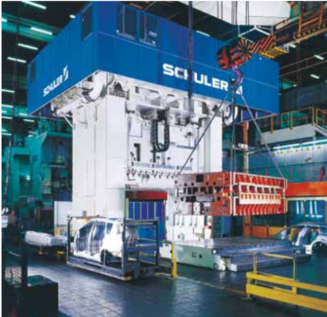
Multicurve-Tryoutpresse zur Simulation aller Pressentypen.
