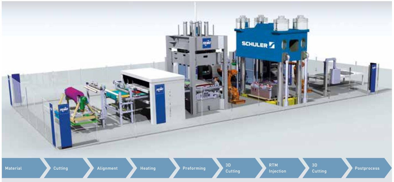
Modular system Production line for RTM components
