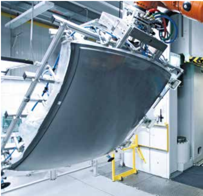
Series production of carbon roofs.
