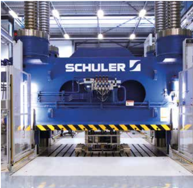
Schuler 36.000 kN short-stroke press for our customer NCC.
