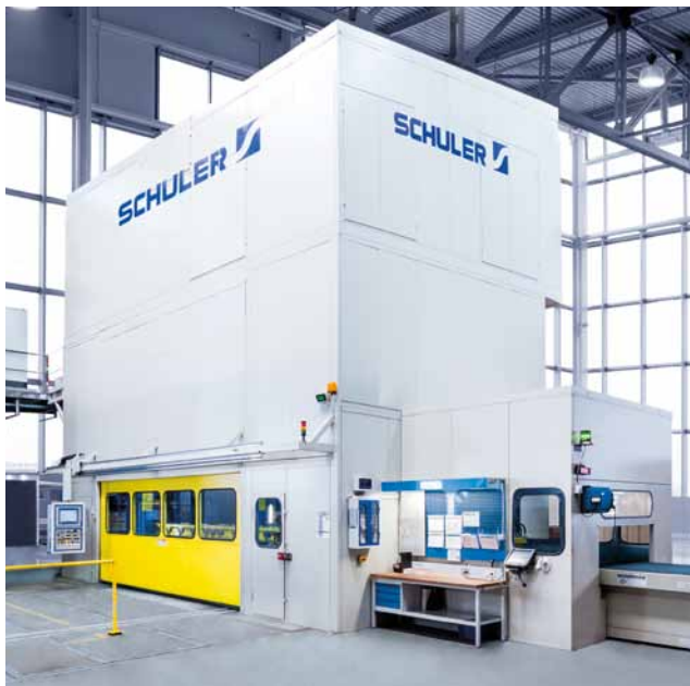
Hydraulic transfer press for flexible parts production.
