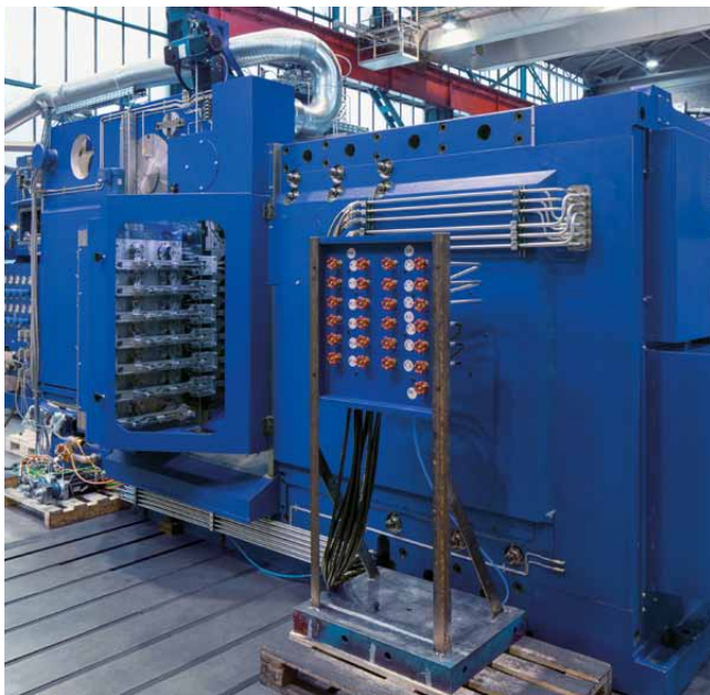
Installation of a FormMaster with ServoDirect technology.
