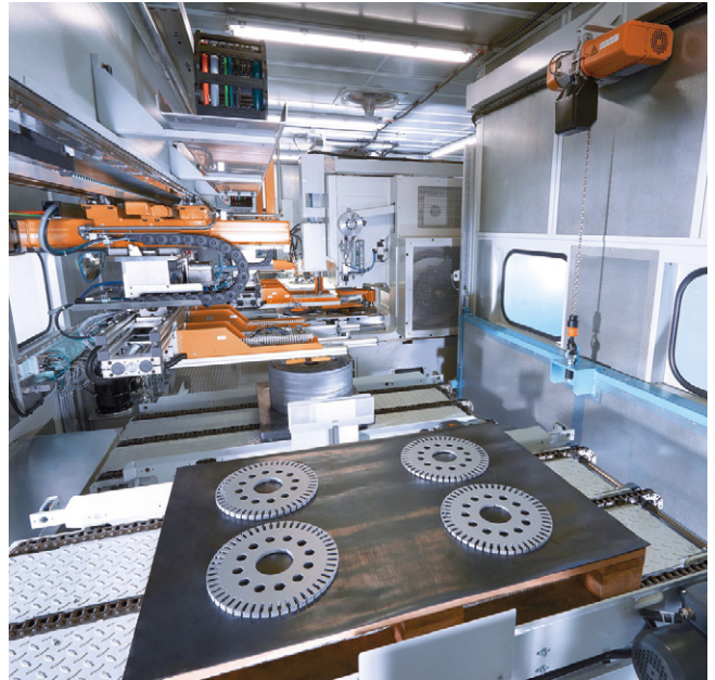
Fully-automated notching line with linear automation.
