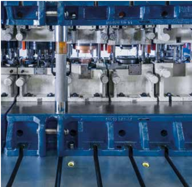
Transfer die for disk holder production.
