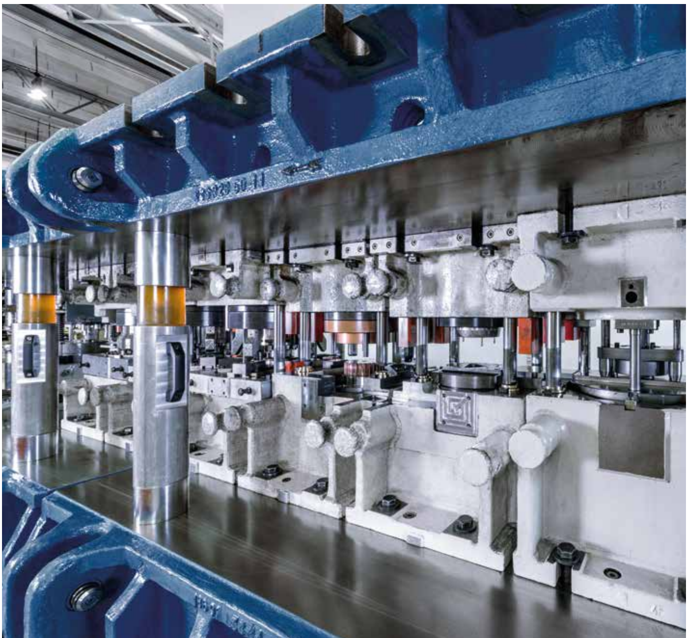
Transfer die for disk holder production.
