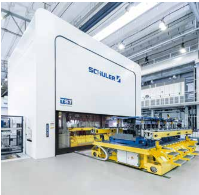
New TST press generation – TwinServo technology at the Servo TechCenter Erfurt.
