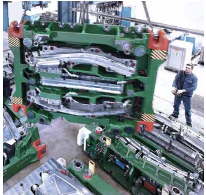
Hot stamping die for the production of high-strength body panel parts.
