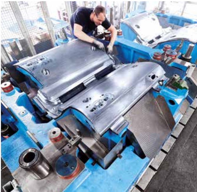
We manufacture dies for cold and hot forming at the Göppingen site.
