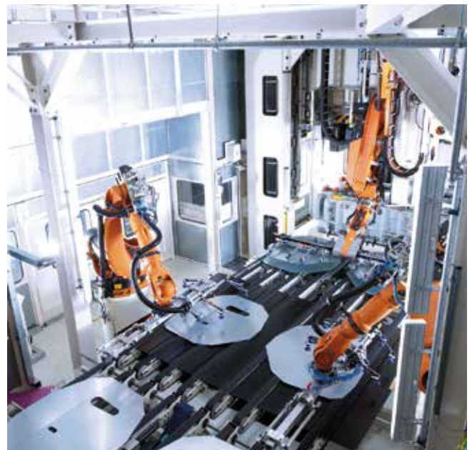
Blankloader of a Schuler servo press line with optical centering station. Press 1 is loaded by a Crossbar Feeder.
