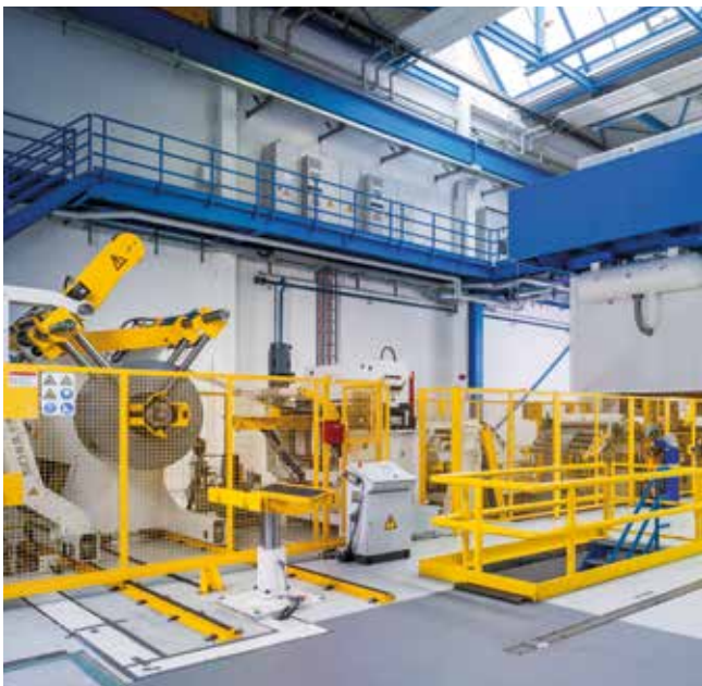
Blanking and forming system with Schuler coil feed line in long space version.
