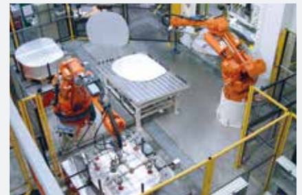
Destacker/blankloader with gravity-type centering station.
