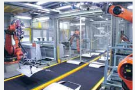
Stacking unit for finished parts.
