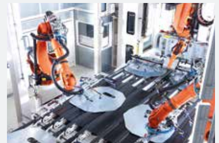
Destacker/blankloader with optical centering station.
