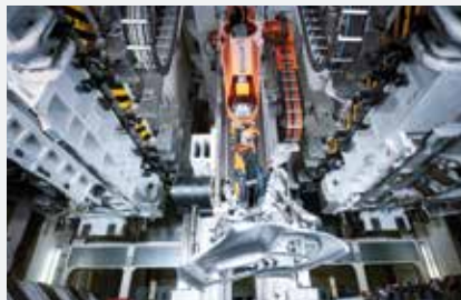
Press line with Crossbar Feeder.
