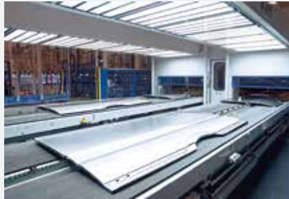
Conveyor for finished parts.
