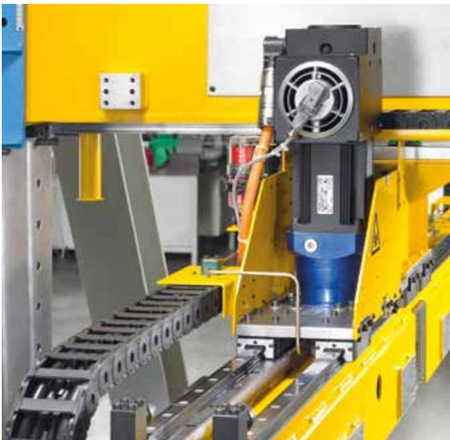
**Direct drive.** The use of direct drives improves accessibility into the press, making the system more maintenance-friendly. Direct drives help customers achieve greater feed increments – up to 3,200 mm (125 in.). They also minimize installation interference with other components such as the feeder, shuttles and conveyors and ensure optimal integration with coil feeding lines and/or destackers/blankloaders.
