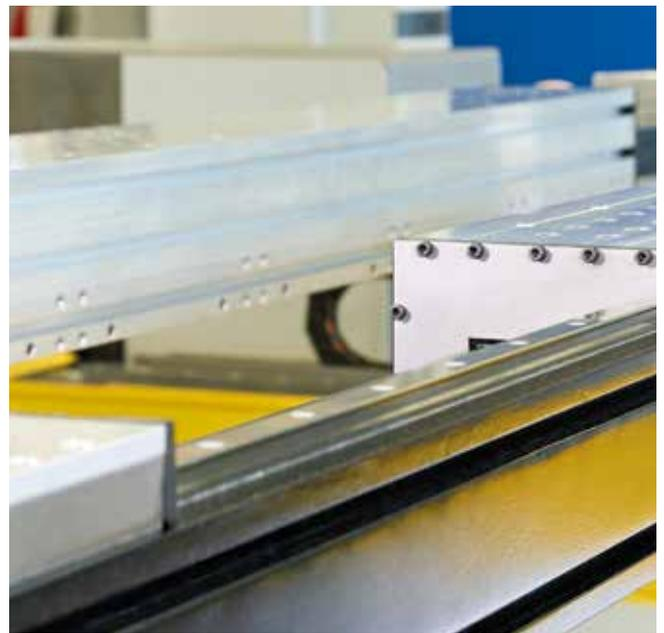
**Linear drive.** The linear drive is only used for the Intra Trans and is integrated into the transfer rails. It enables the compact design and high degree of movement flexibility for this transfer solution.
