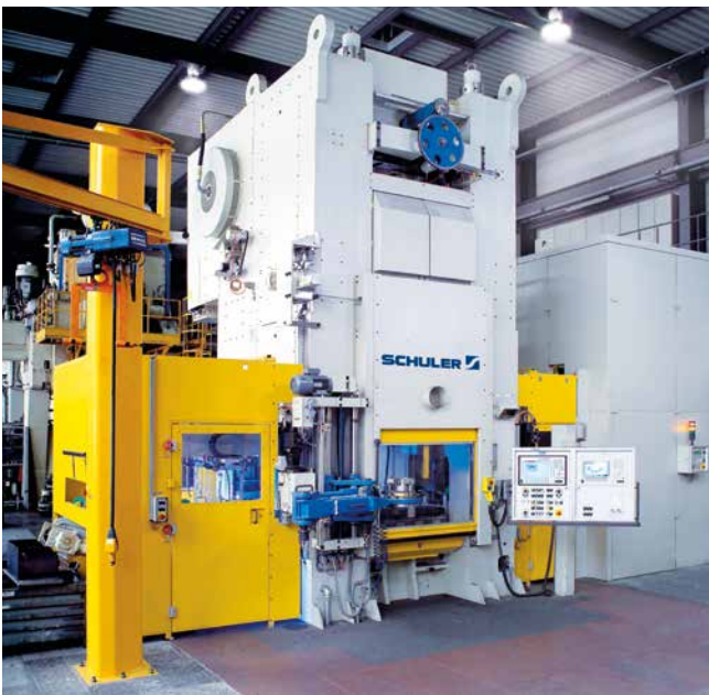
Knuckle joint press with automatic feed, NC transfer system and finished part output.
