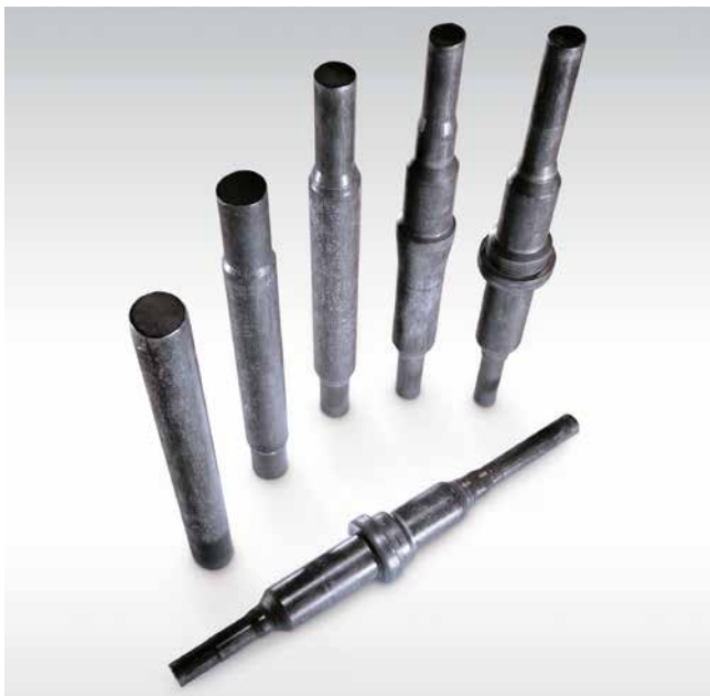
Forming stages of a shaft.
