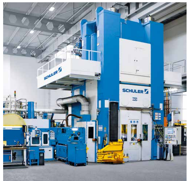
Knuckle joint press with ServoDirect Technology.
