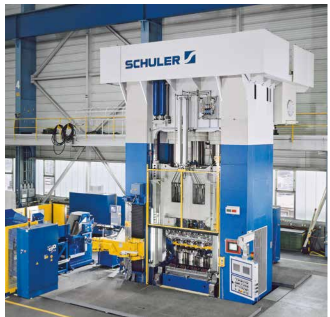
Multi-level hydraulic cold-extrusion press with 16,000 kN press force.
