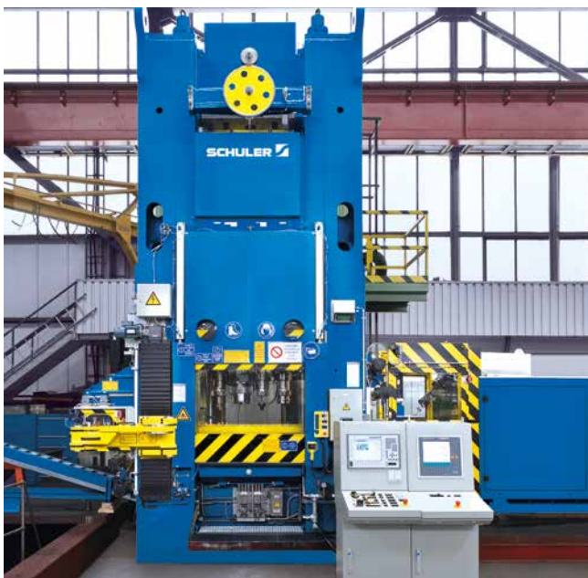
Knuckle joint press with 6,300 kN press force.
