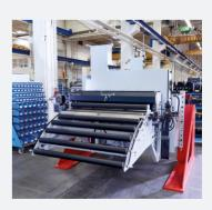
• Power Feed Up to 45 m/s² Coil width 300-1,850 mm
