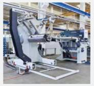
• Long space design Coil thickness 0.5 – 8 mm Coil width 300 – 1,850 mm
