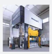
Hydraulic presses HPX series 2,500-8,000 kN
