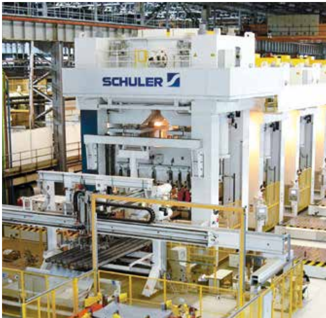
Mechanical high-speed press line with crossbar feeder automation.
