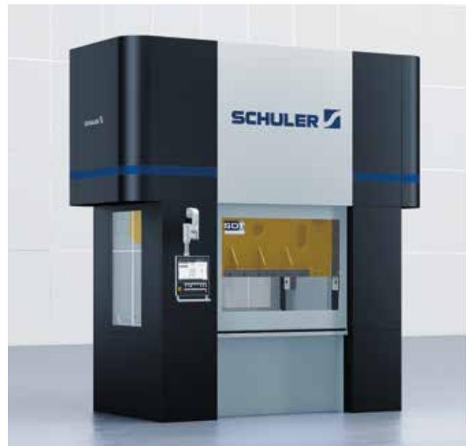
Dual-rod automatic blanking press with MSP 200 ServoDirect technology.
