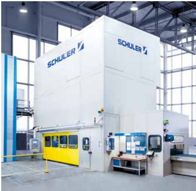
Hydraulic transfer press. Press force: 25 000 kN.
