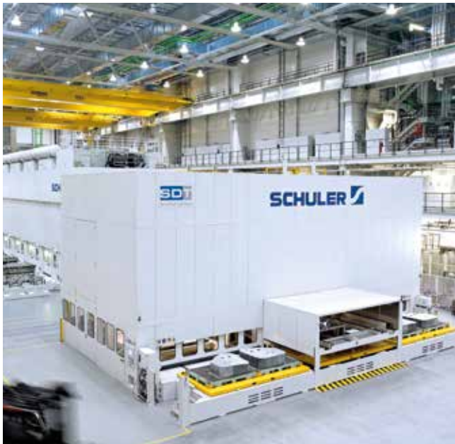
Five-stage press line with ServoDirect Technology and crossbar feeder automation.
