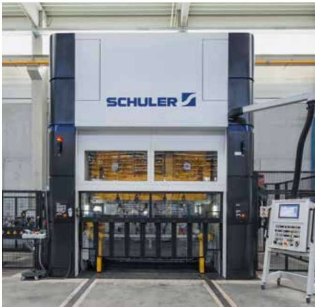
Servo presses in monoblock design with a press force of 400 kN.
