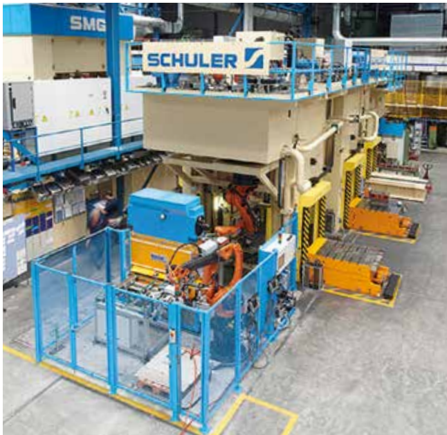
Automated hydraulic press line for manufacturing stainless steel sinks.
