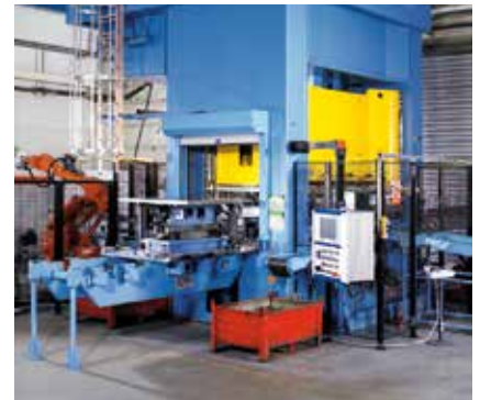
Semi-automatic die change in 15 minutes.
