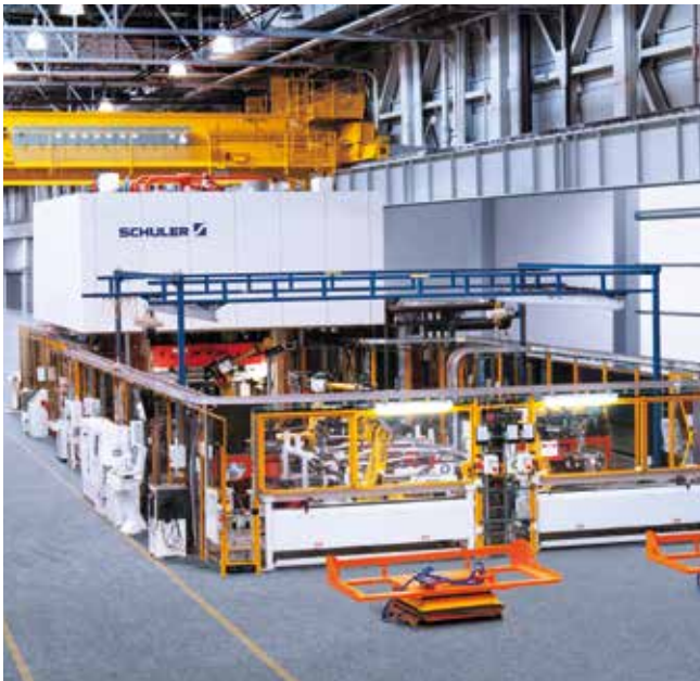
Automated IHU system of an American automobile manufacturer.
