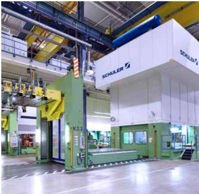
Tryout systems facilitate a highly efficient die run in.
