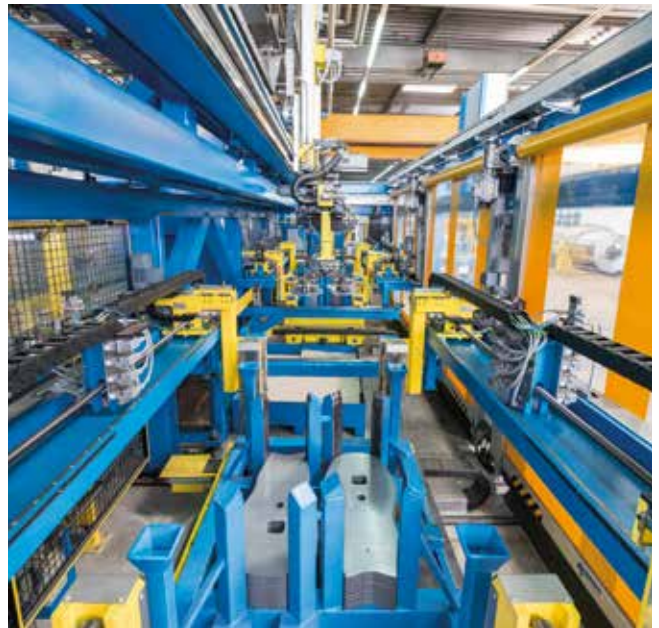
Feeder loading station with blank separation.
