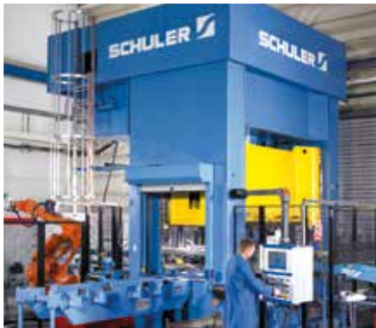
Hydraulic press for the manufacture of side sills and roof braces.
