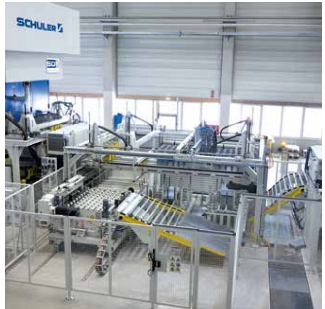
Integrated system solution. Blankloader and coil line on a servo press. Press force: 16 000 kN.
