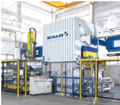
Hydraulic coining press. Press force: 25 000 kN.
