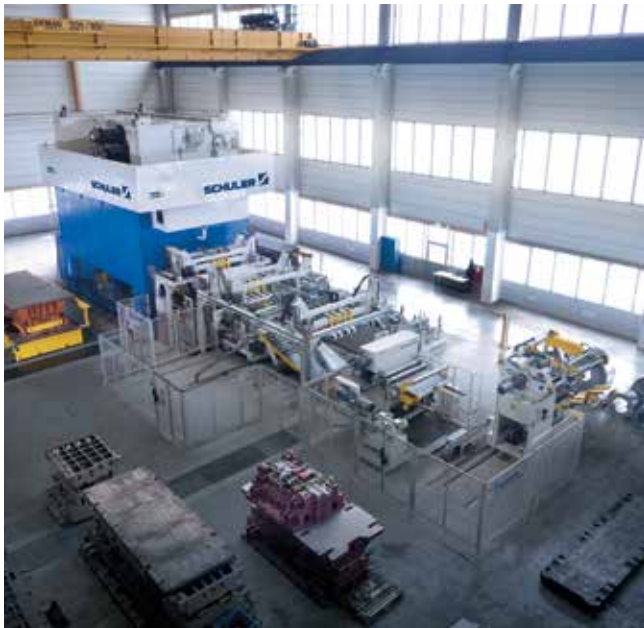
ServoDirect press for cold forming of high-strength steel.
