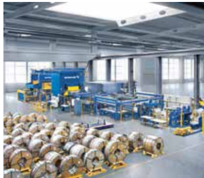
Fully automated production system for the manufacture of heat exchanger plates.
