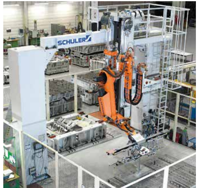
Simulator facility for crossbar feeder.
