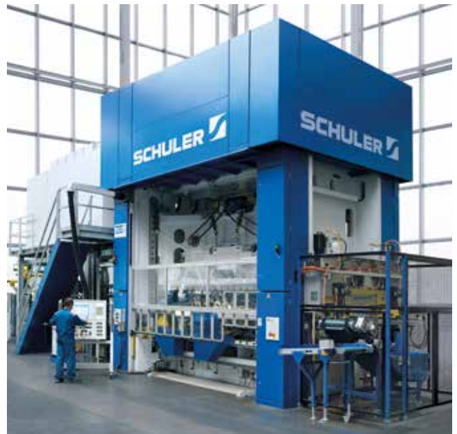
Free programming of the slide movement curves on a servo press with monoblock design and 8 000 kN press force.
