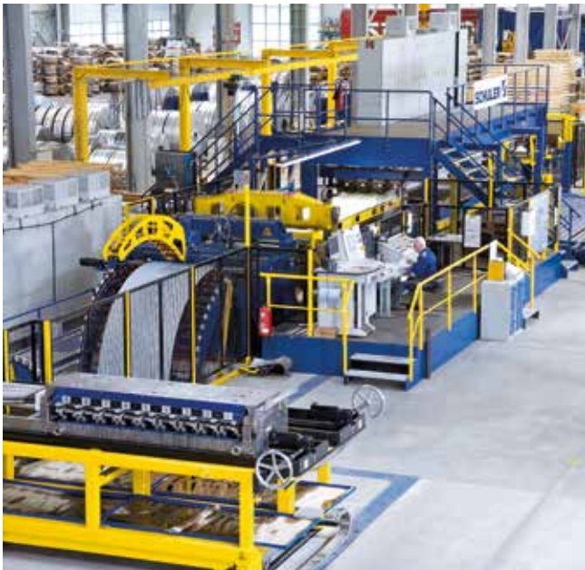
Blanking line with cross-cut shear.
