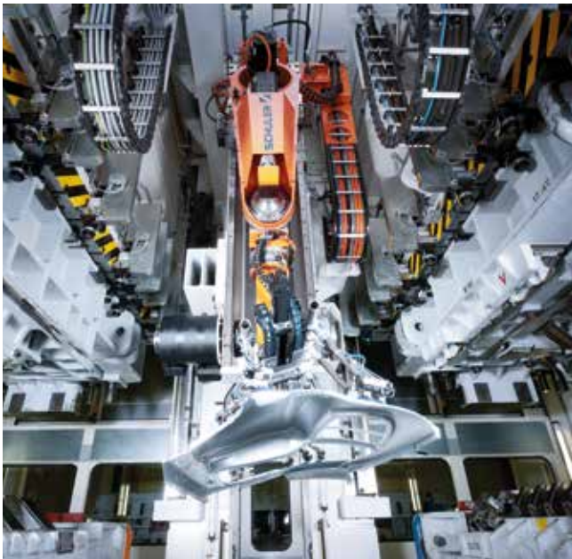
Crossbar feeder within the press line.
