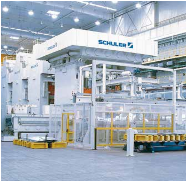
Hybrid press line with hydraulic lead press and mechanical downstream presses.
