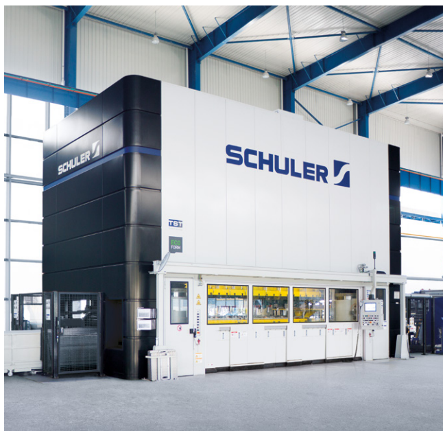
Transfer press with TwinServo technology.
