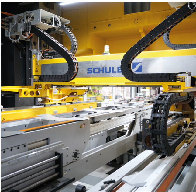
»ProTrans« three-axis transfer system with servo drive.
