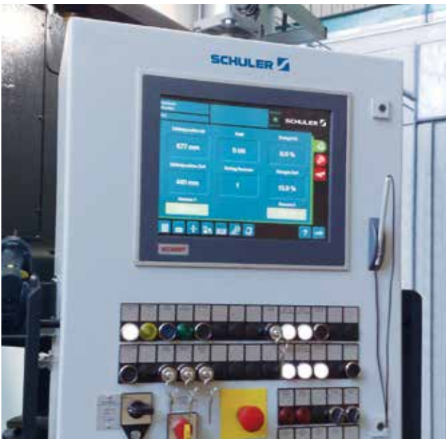
New S7 control component with better visualization and greater ease of use.
