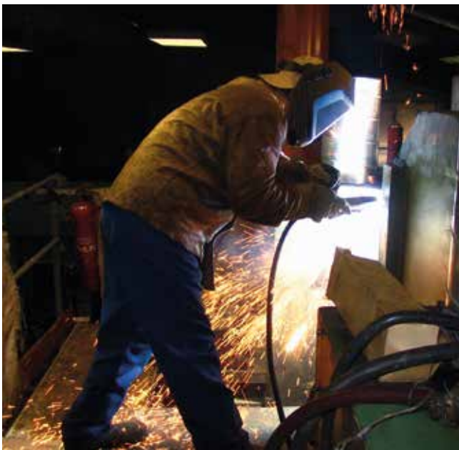
Skilled welders arc gouging to remove a crack in the machine body.
