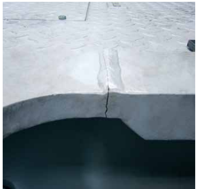
The crack in the slide of a Colombo press was quickly repaired – despite its incomplete technical documentation.
