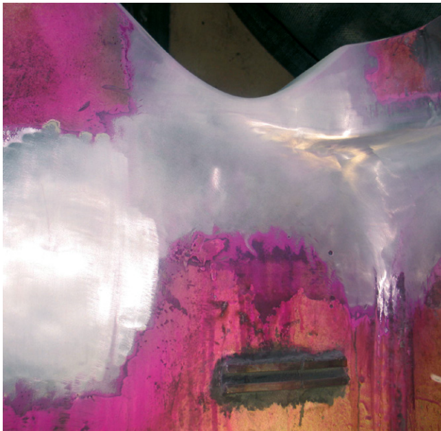
» Repair welding with welded-on and low-notch ground metal transitions.
