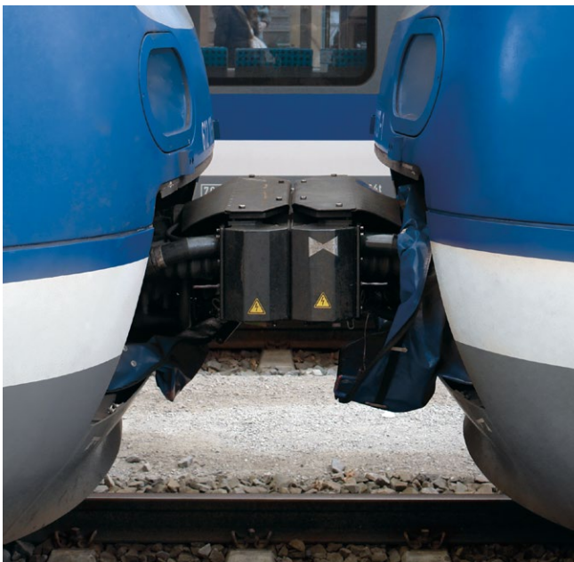
Use of forgings in automatic couplings.
