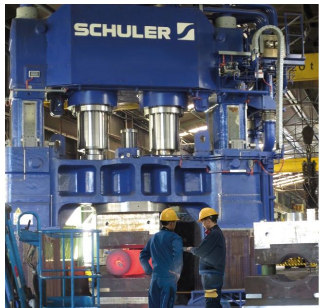
Open die forging press in push down design.
