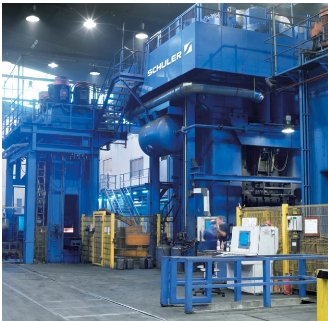
Screw press with hydraulic trimming press on one forging line.
