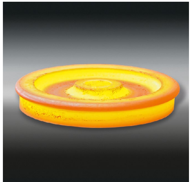
Glowing railway wheel after rolling.
