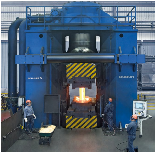
Counterblow hammer with 800 kJ working capacity.
