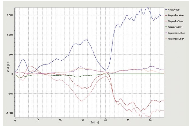
Forces in the sequence of the rolling process.
