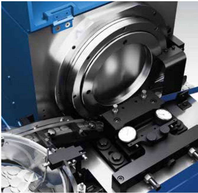
Edge-letting and rimming machine RS 50 for round coin blanks.
