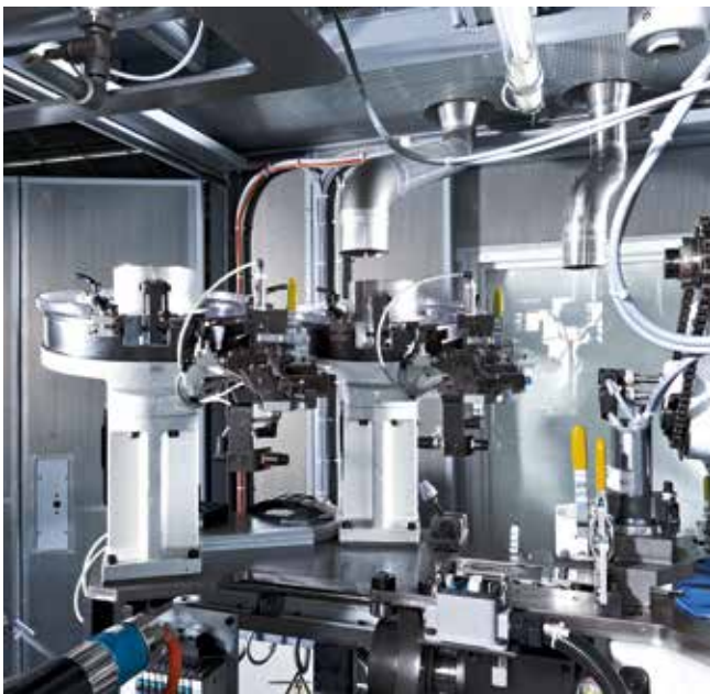
Two feeds for manufacturing bi-metal coins.
