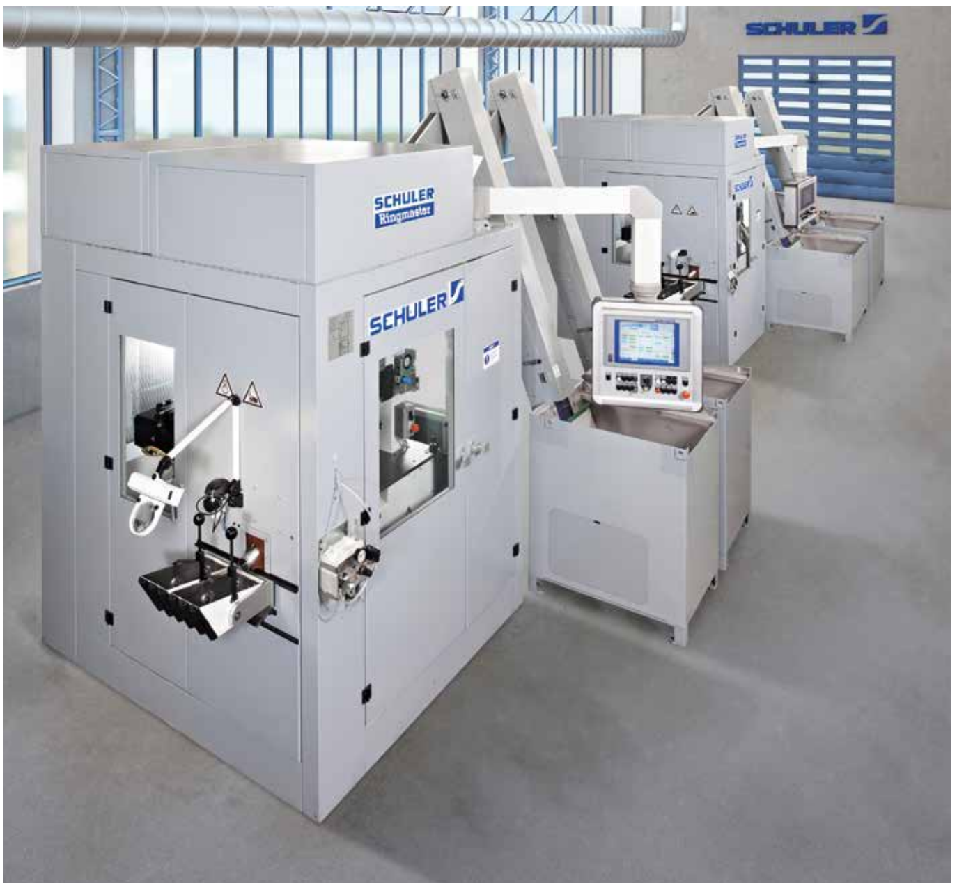
MRV 150 minting presses with Ringmaster equipment.
