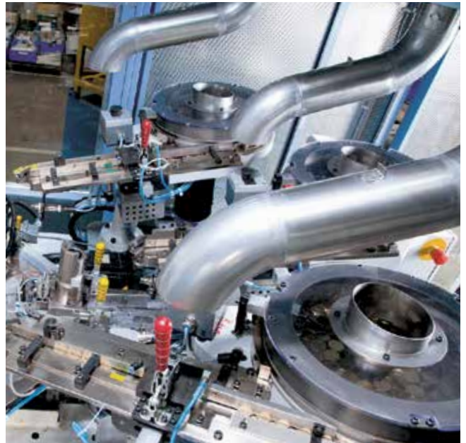
MRV 300 – three feeds for manufacturing a tri-metal coin.
