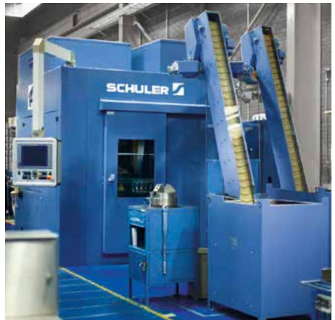
MRV 300 vertical minting press with two feeds.
