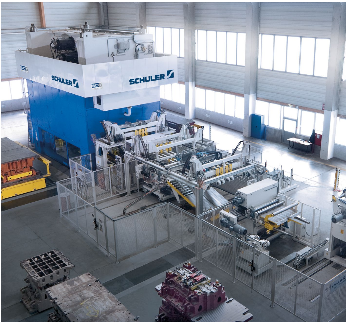
Servo presses in tie rod construction with destacker/coil line combination for manufacturing high-strength structural components.
