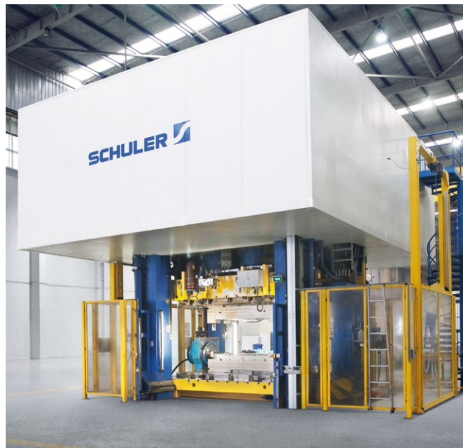
Hydroforming press for high strength and ultra high-strength materials.
