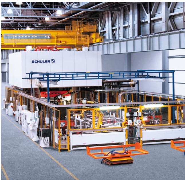
Automated hydroforming line.
