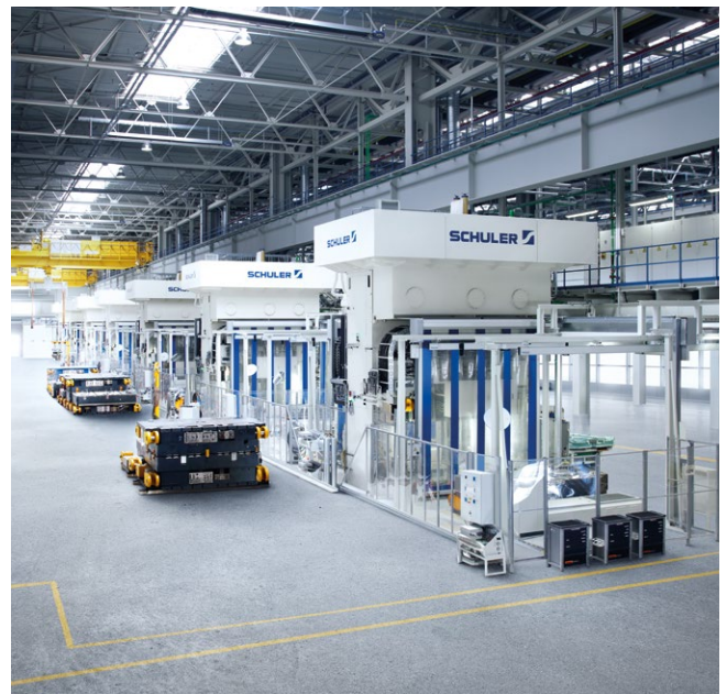
Hydraulic composite molding presses for high volume production.
