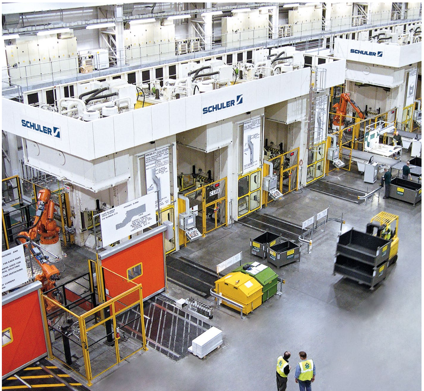
Hydraulic press lines with robot automation for manufacturing aluminum components.
