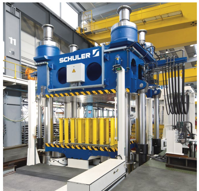
Hydraulic short stroke press for producing fiber-reinforced plastics.
