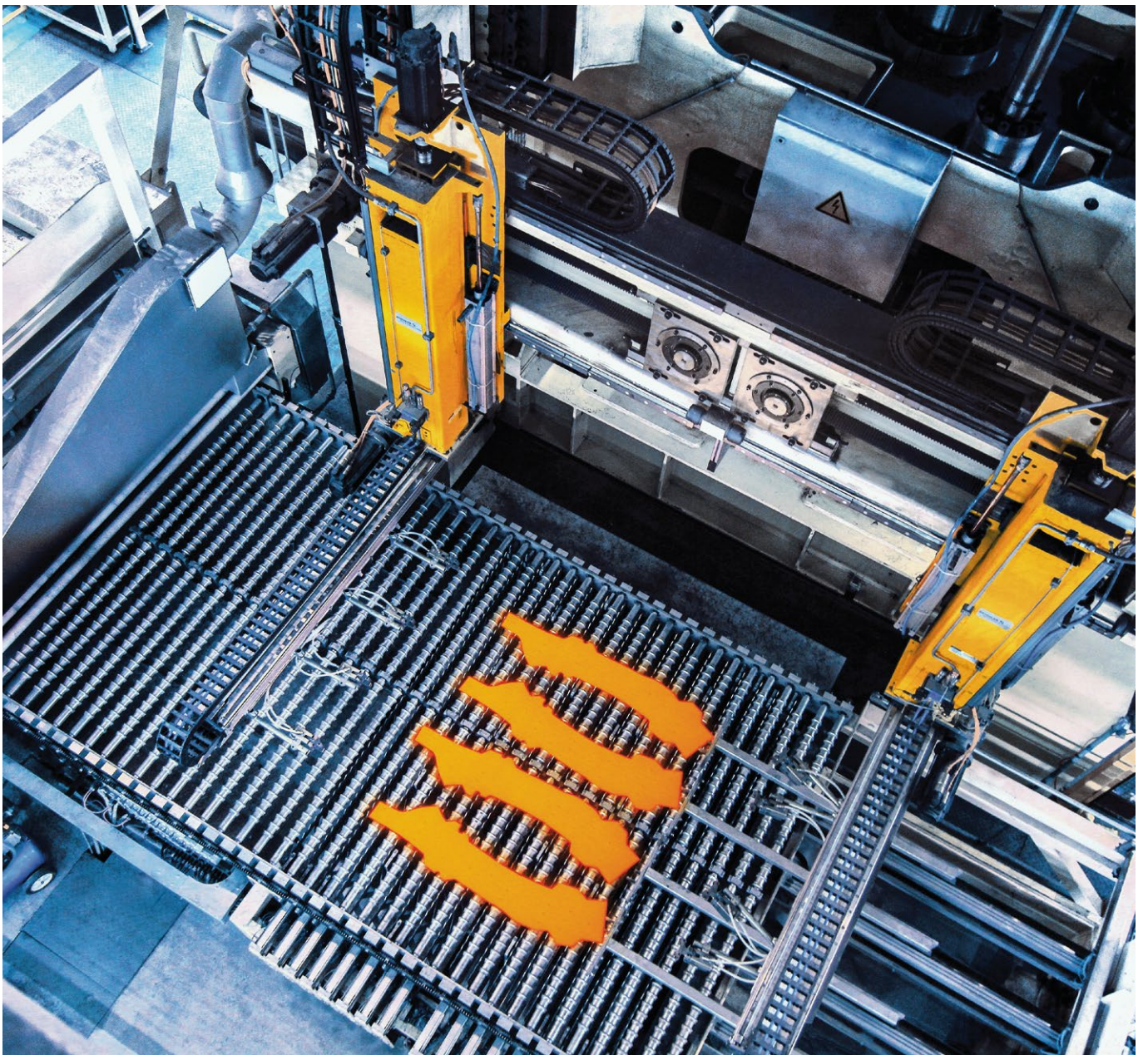
Hot Stamping in series production with PCH Technology.
