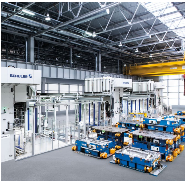
Hydraulic composite molding presses for high volume production.
