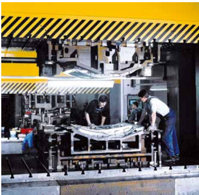
Hydraulic tryout presses are the key to fast die start-up.
