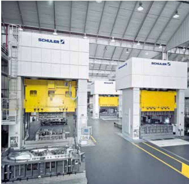
Tryout center with hydraulic tryout presses.
