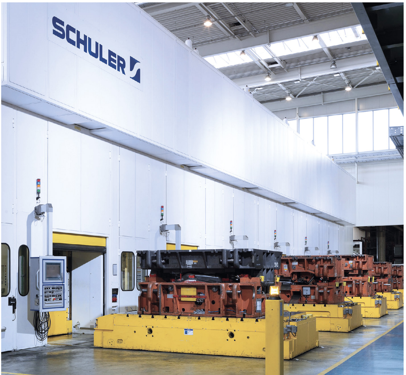
Hydraulic press line with Crossbar Robot automation. Total capacity: 66.000 kN (6 presses).
