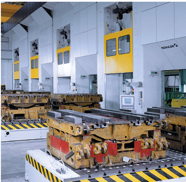
Fully automatic die change system.
