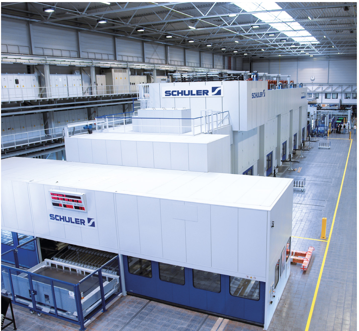
Hydraulic press line with Schuler blankloader and robot automation. Total press force: 89.000 kN (five presses).
