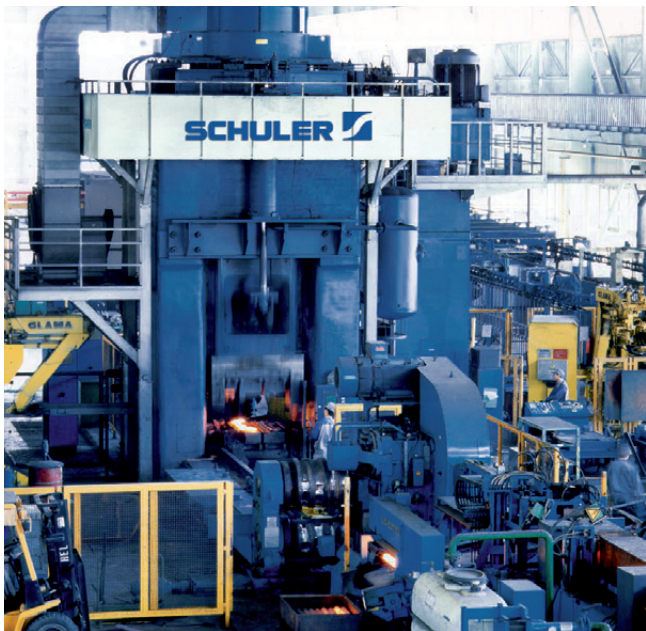
Screw press type PSH 4.630f for manufacturing parts for light trucks.
