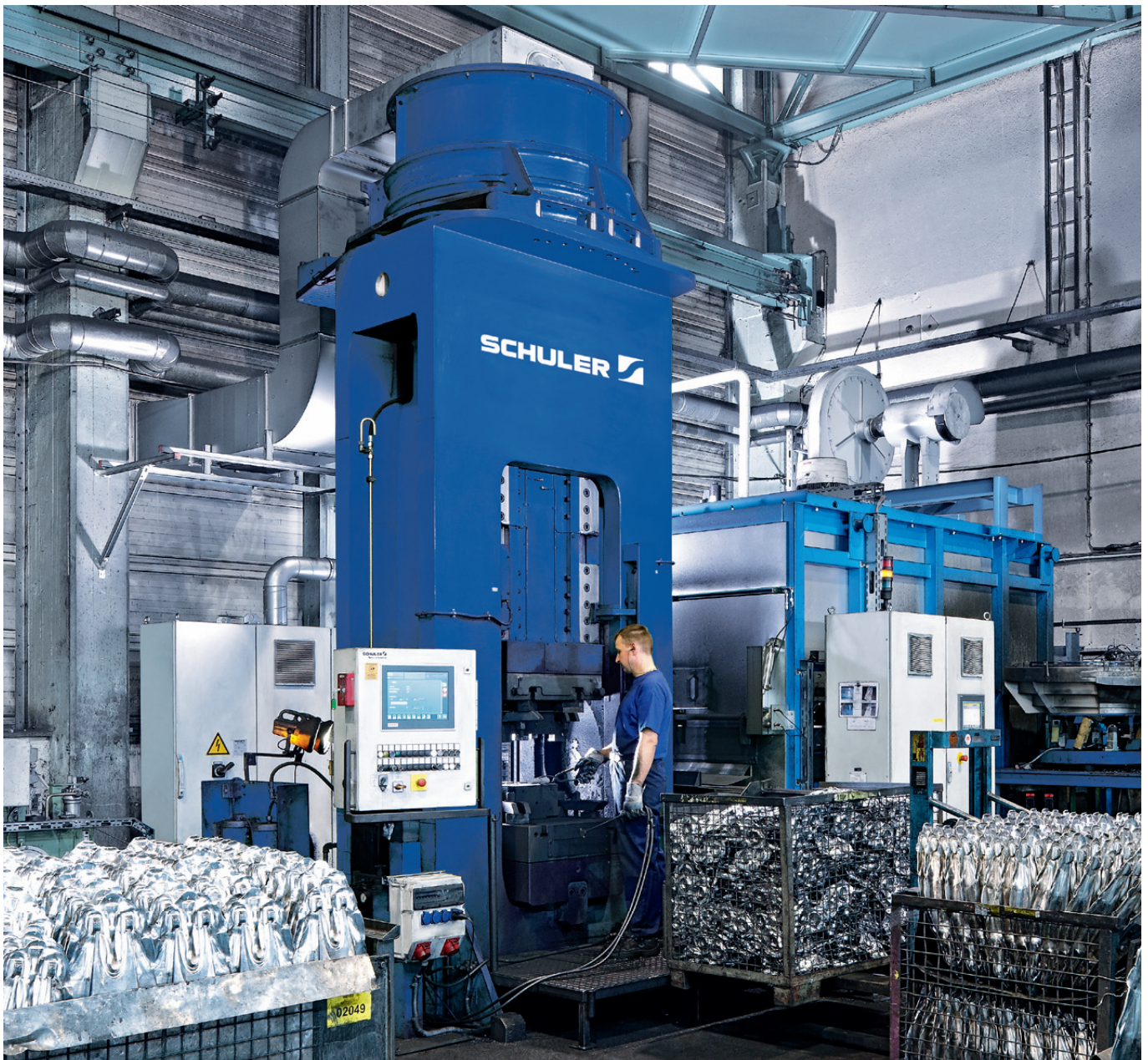
Screw press type PAR265f for manufacturing aluminum forgings.
