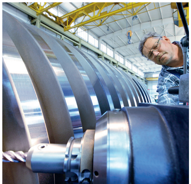
A Schuler Group employee machining the profile for the screw of a screw press.
