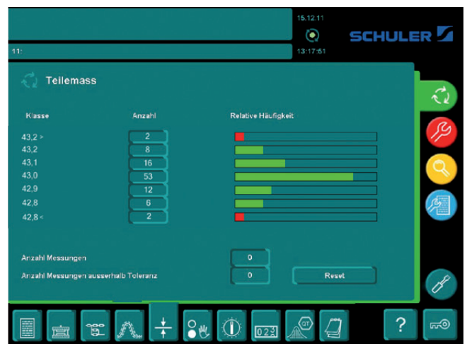
Thickness measurement including Gaussian standard distribution curve.
