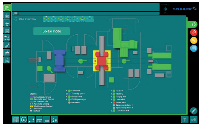
Forge Control System for monitoring the complete forging line.
