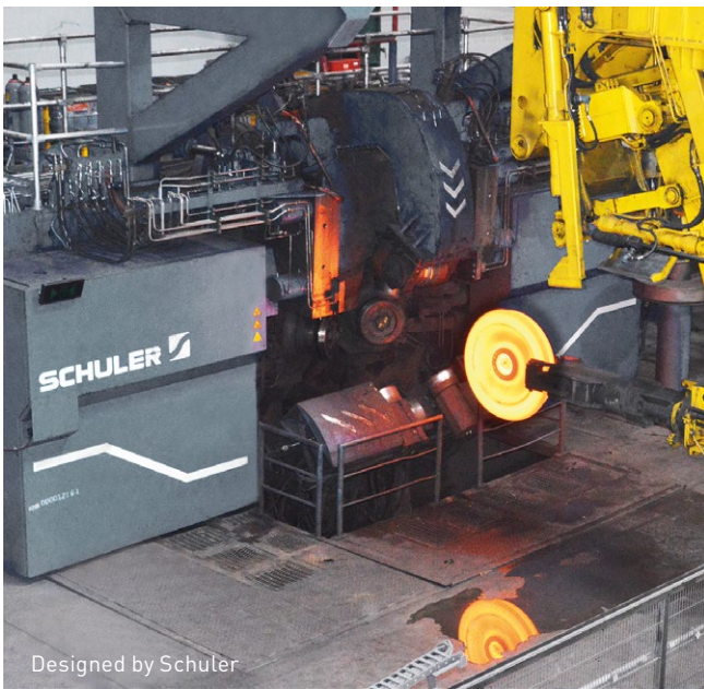
Schuler wheel roller optimized for extended tool life.
