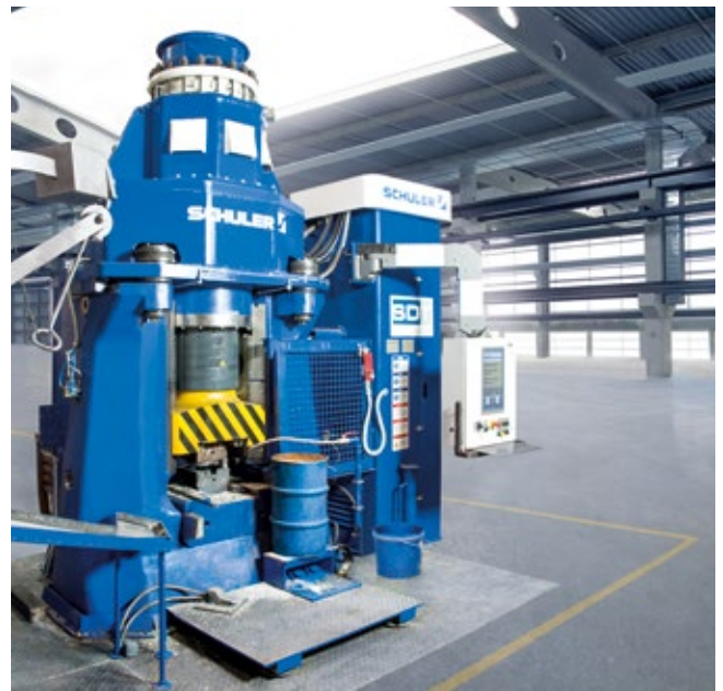
Linear hammer with ServoDirect technology.
