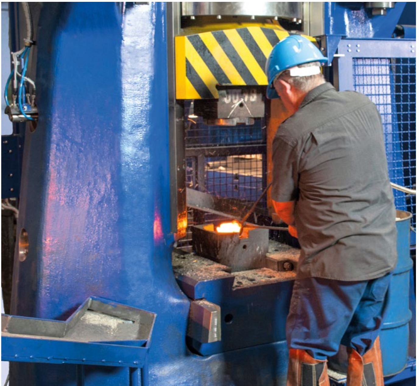
Linear hammer used for forging.
