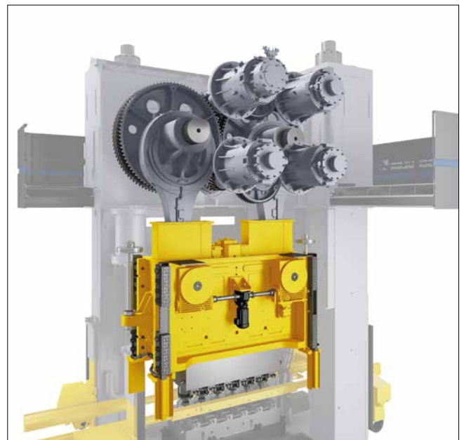
Drive of MSE press with four torque servo motors.
