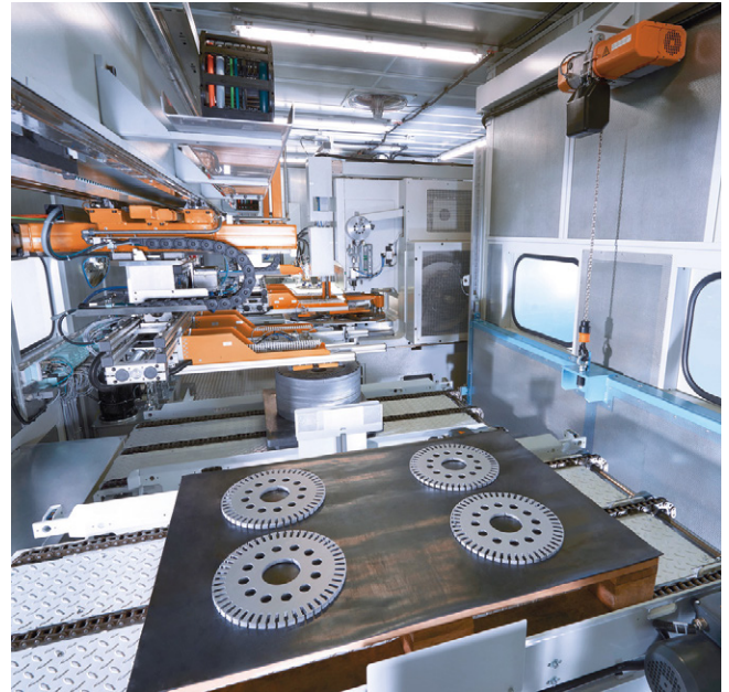
Fully-automated notching line with linear automation.
