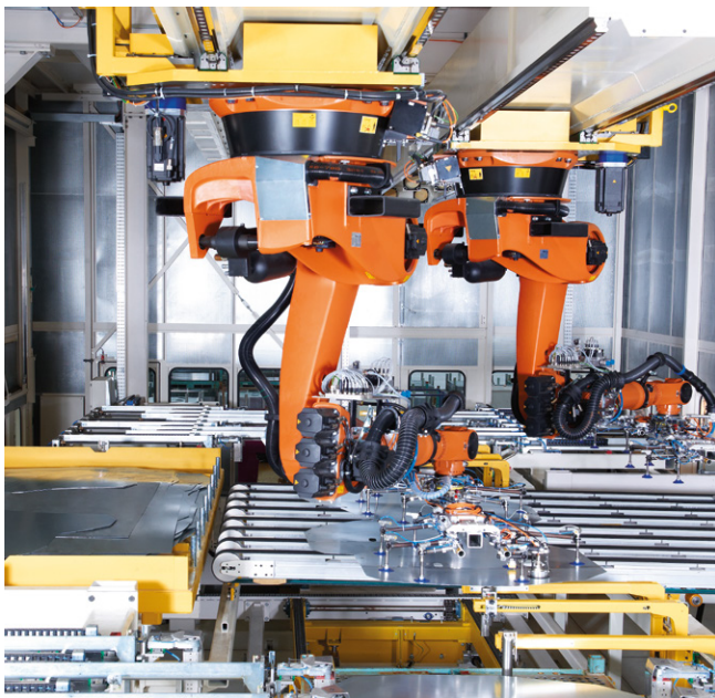
Destacking the blanks. Two robots from Schuler suspended on linear axes alternately destack the blanks and reliably deposit them on a conveyor belt.
