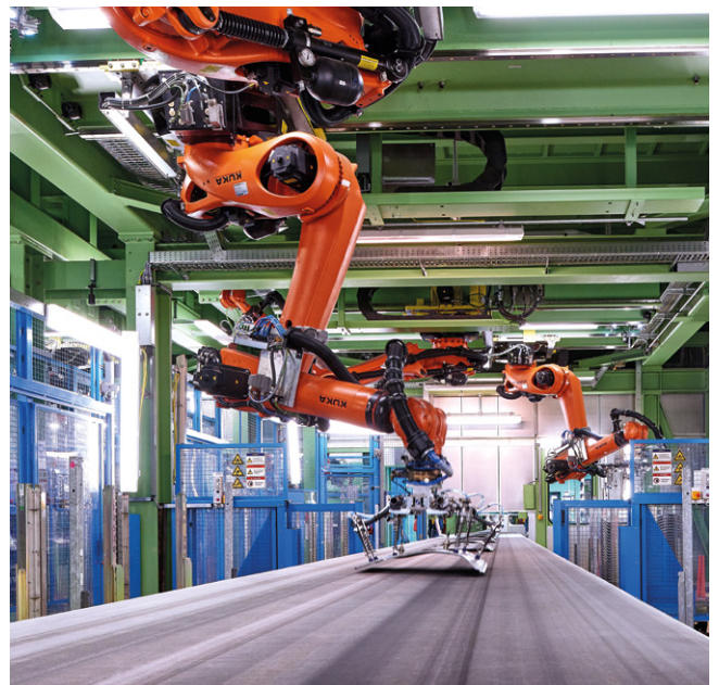
Robots pick up the finished parts from the belt and put them into storage.
