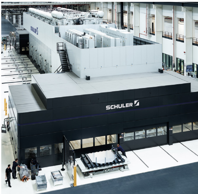
Six-stage press line with ServoDirect Technology and Crossbar Feeder automation.
