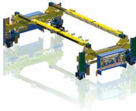
Example 2: Schuler Intra Trans, AT2 model with a support width of 4,200 mm and a drive unit width of 1,800 mm. Fitted with carbon and aluminum rails for the use in a ProgDie press.
