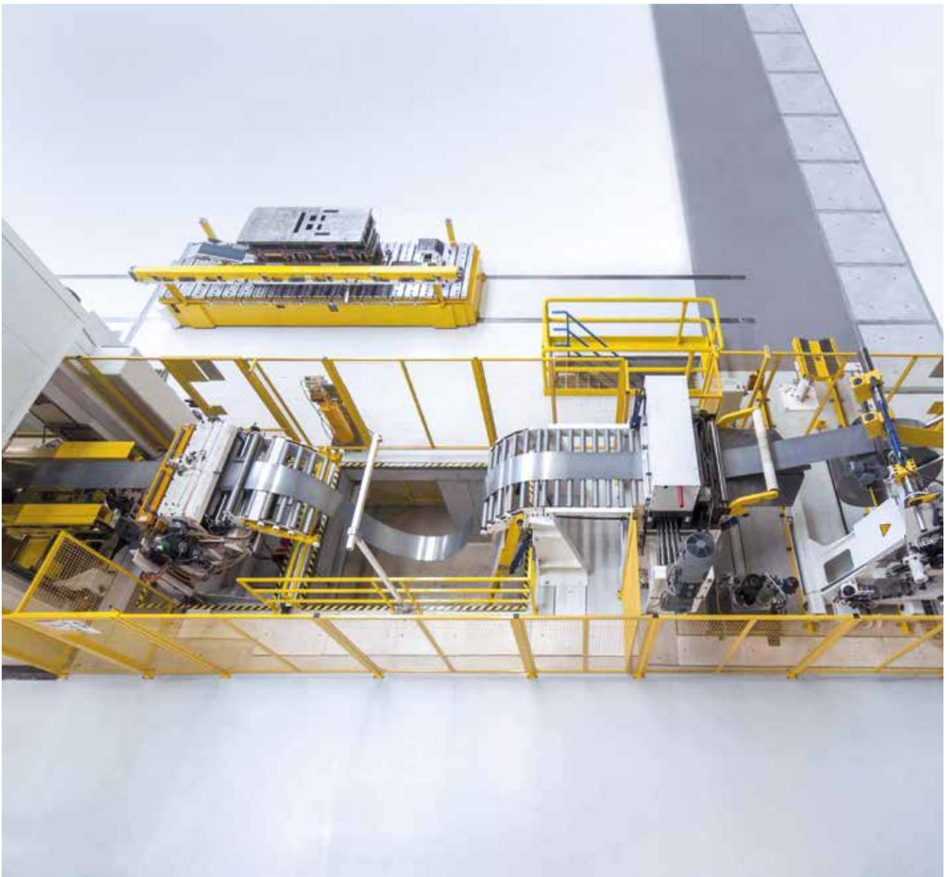
Coil feeding line-in long-space design with roll feed and zig-zag option for optimized use of material.
