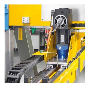
Direct drive. The use of direct drives improves accessibility into the press, making the system more maintenancefriendly. Direct drives help customers achieve greater feed increments – up to 3,200 mm (125 in.). They also minimize installation interference with other components such as the feeder, shuttles and conveyors and ensure optimal integration with coil feeding lines and/or destackers/blankloaders.
