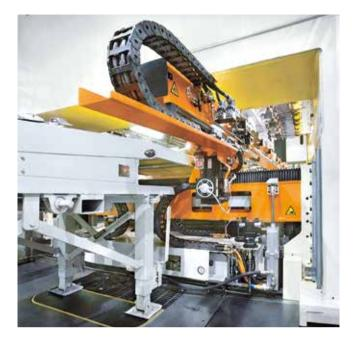
Transfer retrofit. Schuler tri-axis transfers are well suited for all types of lines by any press supplier. The installation of a new transfer is an effective and cost-efficient way to modernize existing lines – doing away with often expensive and time-consuming maintenance for older mechanical transfers. Reliability, precision and throughput capacity are significantly improved. Schuler tri-axis transfers have short delivery times and can be easily integrated into your presses.
