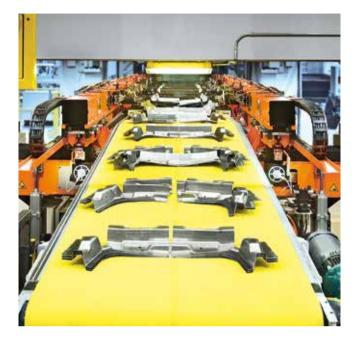
Wide range of applications. The available capacities are designed for use on presses with bed sizes of up to 8,100 × 3,100 mm (319 × 122 in.). The applications range from smaller parts such as seat rails and axle brackets up to doors and hoods. The very rigid yet lowmass and low-inertia design of the new tri-axis transfer permits extremely high stroke rates and short changeover times, especially in the manufacture of smaller parts.
