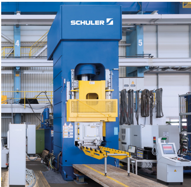
6,300 kN Isothermal forming press with integrated heat chamber.
