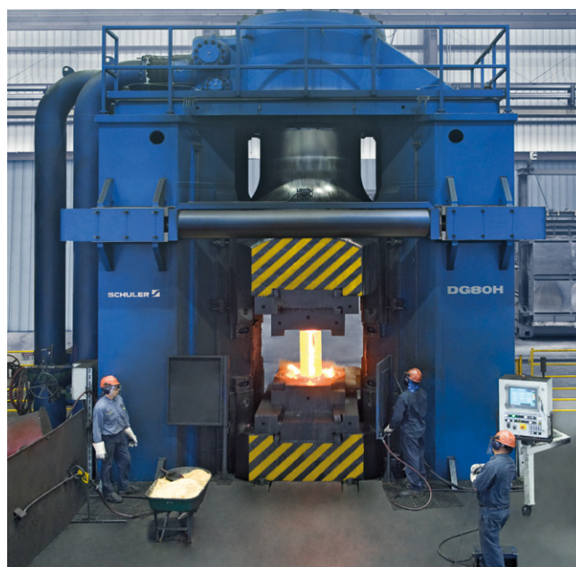
Counterblow hammer with 800 kJ working capacity.
