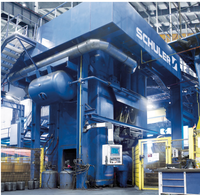
Screw press with direct drive PZ S 900f with 128,000 kN press force for manufacturing heavy forgings.
