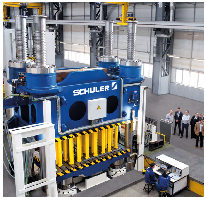
Hydraulic press for manufacturing fiber-reinforced plastics at Schuler.
