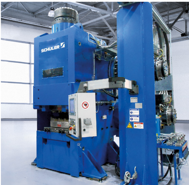
The upsetter with ServoDirect Technology manufactures pre-forms for compressor blades.
