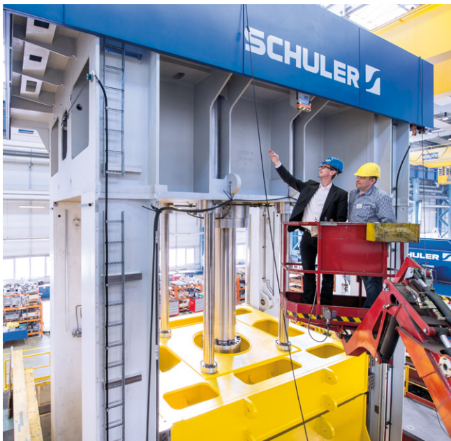
Hydraulic press for manufacturing individual parts for booster rockets used in civil spaceflight.
