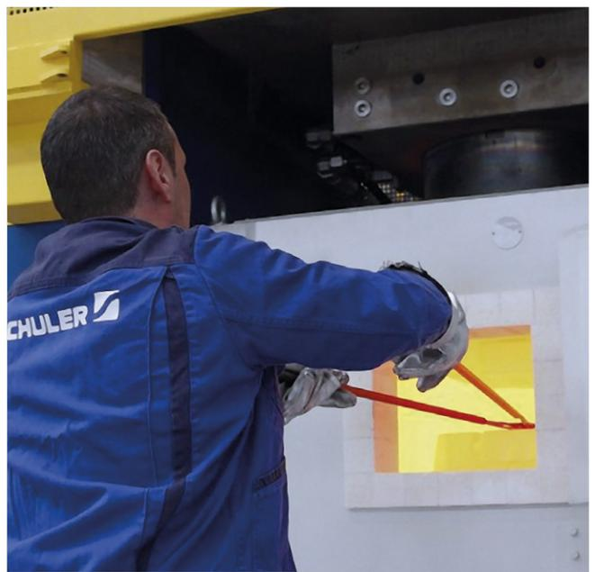
Wärmekammer in Isotherm-Umformpresse.
