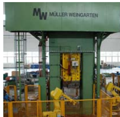
Screw press with a max. press force of 3,200 metric tons (3,520 US tons)
