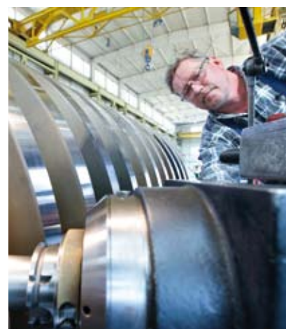
A Schuler Group employee working on the thread of a forging press screw
