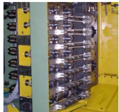
Transfer system for six stations with depositing gripper
