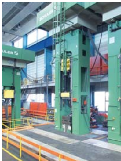
Line with three hydraulic presses for manufacturing CNG tanks
