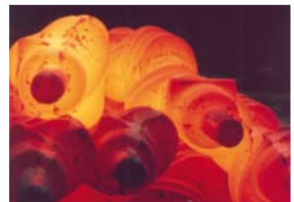
A crankshaft is finished in only 50 seconds
