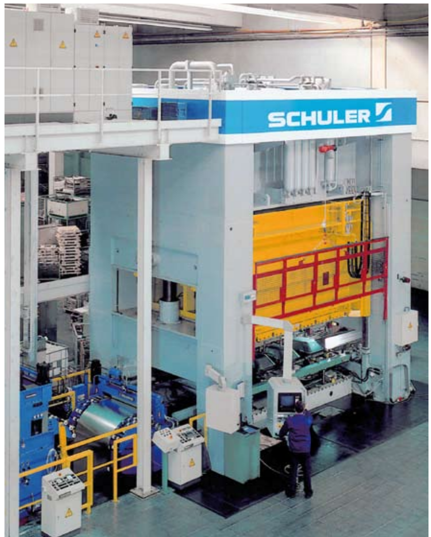
Hydraulic transfer press with a capacity of 12,000 kN.
