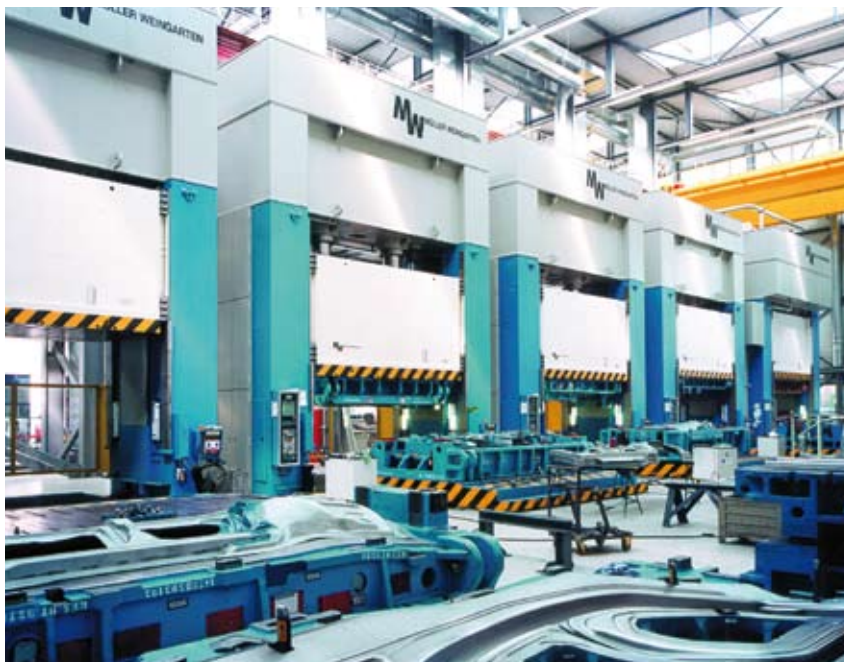
Tryout center with hydraulic tryout and multicurve presses.
