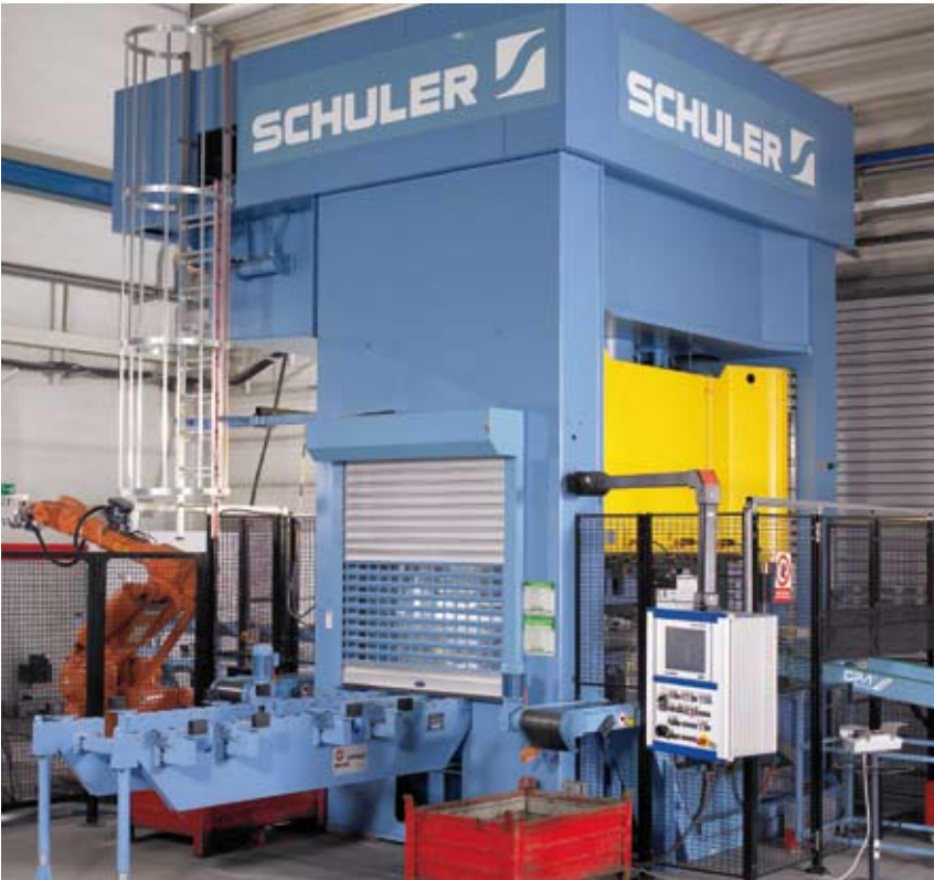
Hydraulic single press. Schuler's SH-series for hydraulic single presses ranges from 1,600 up to 16,000 kN.
