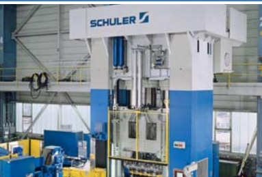
Hydraulic cold extrusion presses
