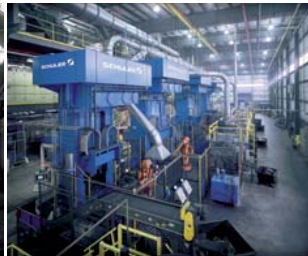
Hydraulic presses for forging aluminum wheels
