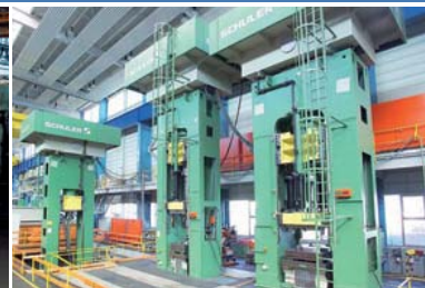
Hydraulic presses for manufacturing CNG gas cylinder tanks
