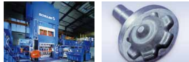
MME-series, 3,150–31,500 kN / MSE-series with servo drive
