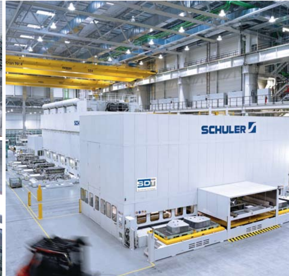
Servo press line with Schuler blankloader, Crossbar Feeder automation and end-of-line system.
