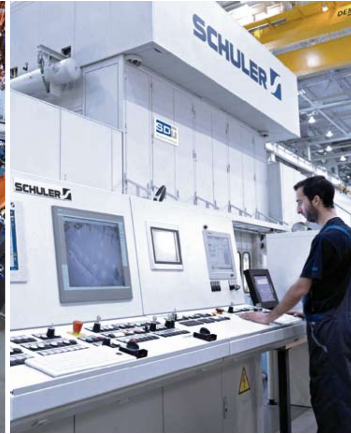
Main control panel of a blanking line with ServoDirect Technology.
