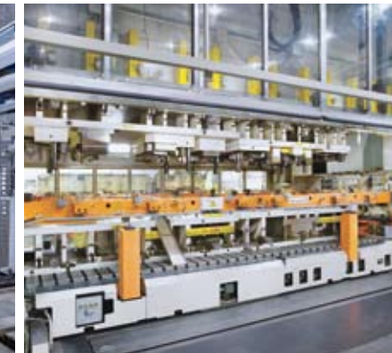
6. Modular electronic three-axis transfer.
