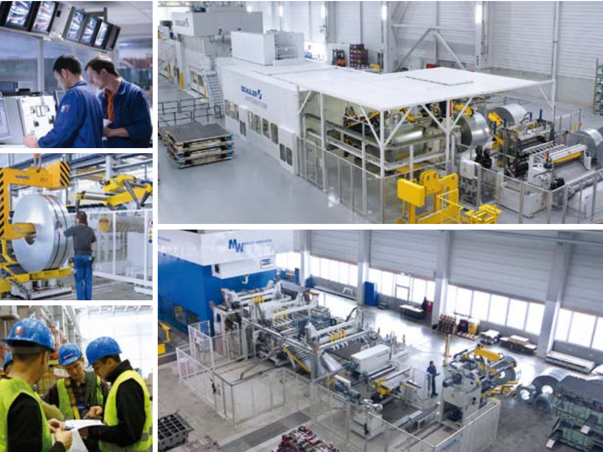
Servo press with combination of coil feed line and blankloader.
