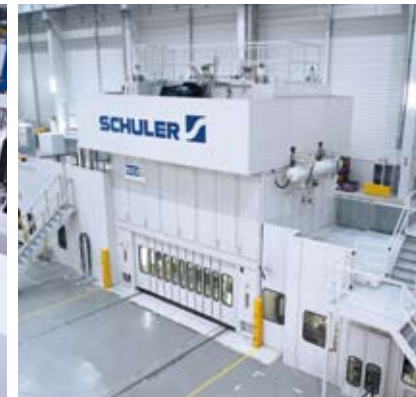
5. Blanking press with ServoDirect Technology.
