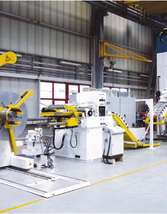
Blanking and forming system with Schuler coil feed line in long space version.
