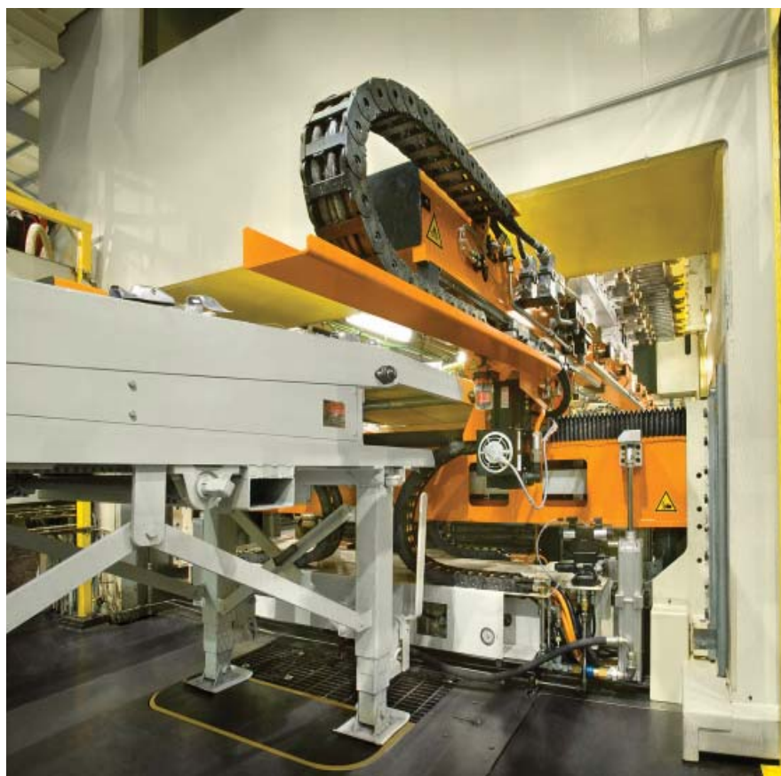
Schuler transfer retrofit installed in a Verson press. Compact and flexible mounting design fits within existing system.
