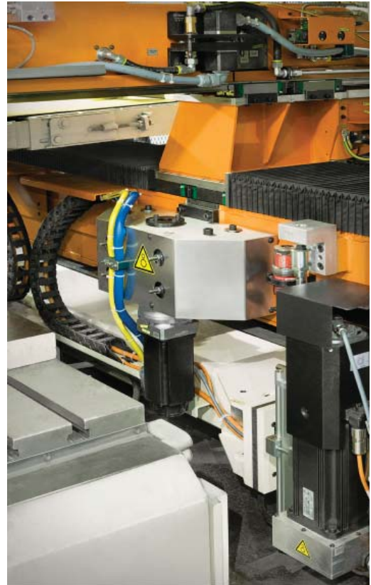
Designed with direct drives, reciprocating mass in the system is reduced.
