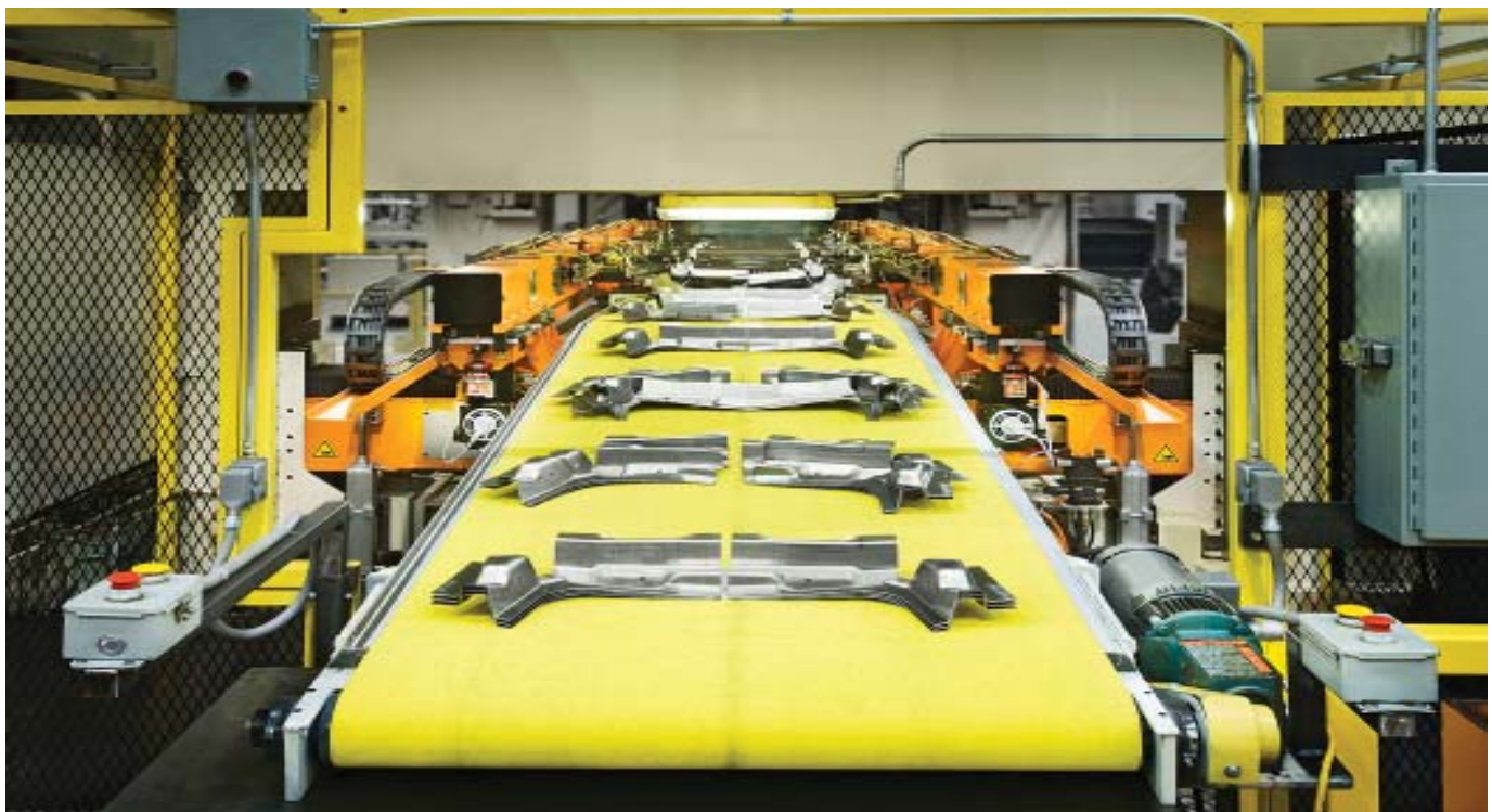
A newly developed transfer rail guide improves the rigidity of the AT transfer, allowing high stroke rates while maintaining consistent quality.
